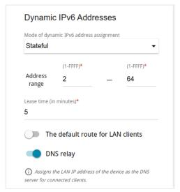
Figure 90. Configuring the local interface. The IPv6 tab. The Dynamic IPv6 Addresses section.
