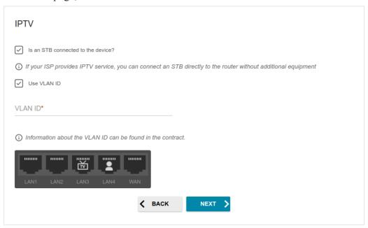
Figure 49. The page for selecting a LAN port to connect an IPTV set-top box.
