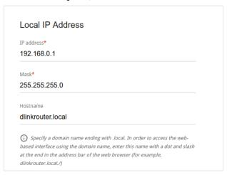
Figure 82. Configuring the local interface. The IPv4 tab. The Local IP Address section.
