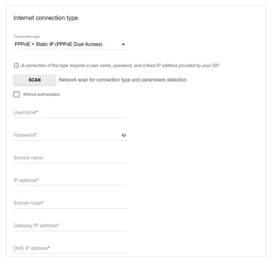
Figure 44. The page for configuring PPPoE + Static IP (PPPoE Dual Access) WAN connection.
