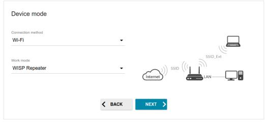
Figure 35. Selecting an operation mode. The WISP Repeater mode.
