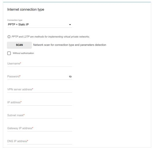
Figure 46. The page for configuring PPTP + Static IP WAN connection.
