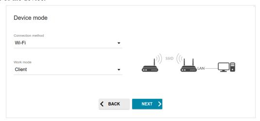
Figure 38. Selecting an operation mode. The Client mode.
