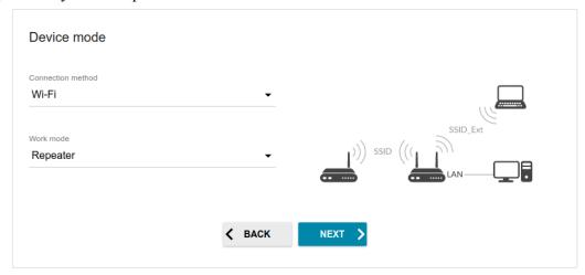
Figure 37. Selecting an operation mode. The Repeater mode.
