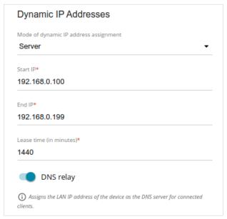
Figure 83. Configuring the local interface. The **IPv4** tab. The **Dynamic IP Addresses** section.
