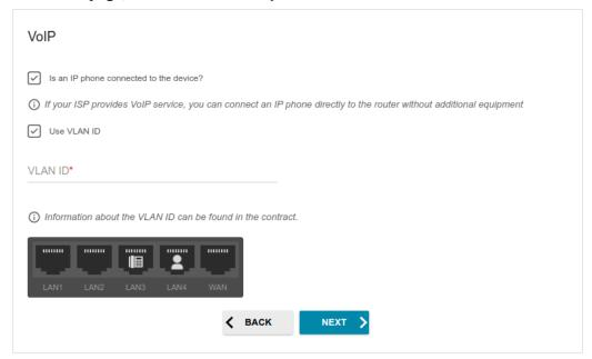
Figure 50. The page for selecting a LAN port to connect a VoIP phone.
