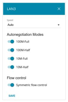
Figure 119. The window for changing the settings of the router's port.
