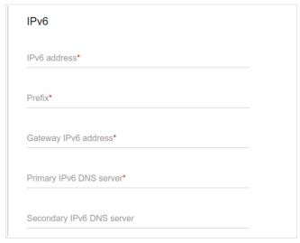
Figure 69. The page for creating a new **Static IPv6** connection. The **IPv6** section.
