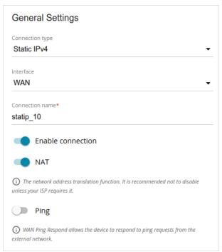
Figure 64. The page for creating a new Static IPv4 connection. The General Settings section.
