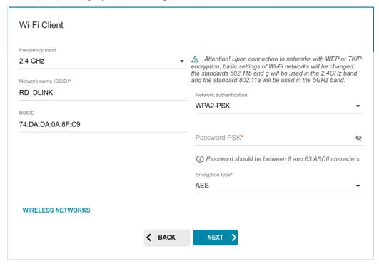
Figure 40. The page for configuring the Wi-Fi client.
