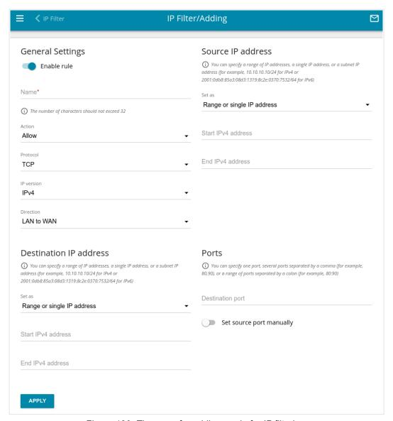
Figure 130. The page for adding a rule for IP filtering.
