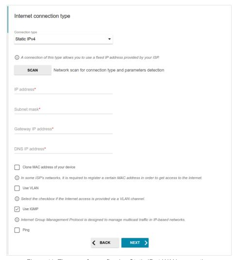
Figure 41. The page for configuring Static IPv4 WAN connection.
