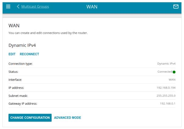
Figure 62. The Connections Setup / WAN page. The simplified mode.
