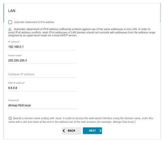
Figure 39. The page for changing the LAN IPv4 address.
