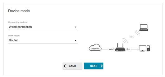
Figure 34. Selecting an operation mode. The Router mode.
