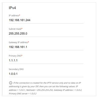
Figure 66. The page for creating a new Static IPv4 connection. The IPv4 section.
