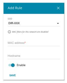
Figure 108. The window for adding a rule for the MAC filter.
