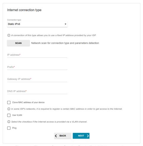
Figure 42. The page for configuring Static IPv6 WAN connection.
