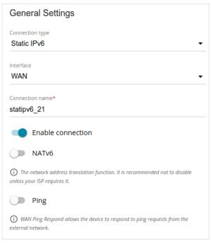
Figure 67. The page for creating a new Static IPv6 connection. The General Settings section.
