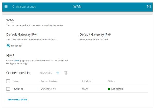
Figure 63. The Connections Setup / WAN page. The advanced mode.
