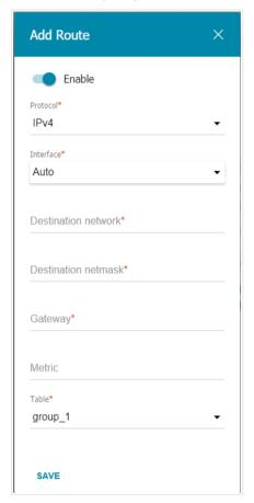
Figure 122. The window for adding a new route.
