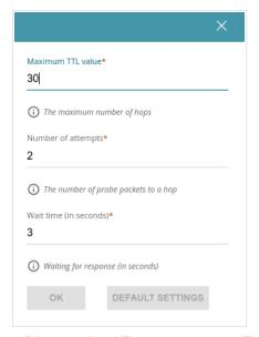
Figure 141. The Management / Diagnostics / Traceroute page. The additional settings window.
