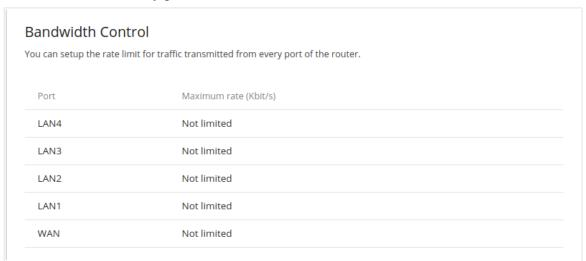
Figure 117. The Functions / Advanced / Bandwidth Control page.
