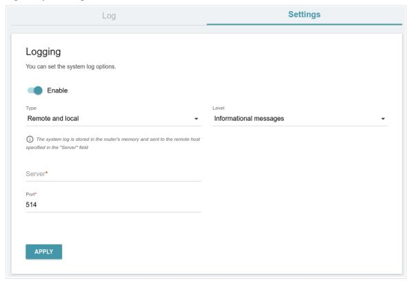
Figure 125. The Management / System Log page. The Settings tab.
