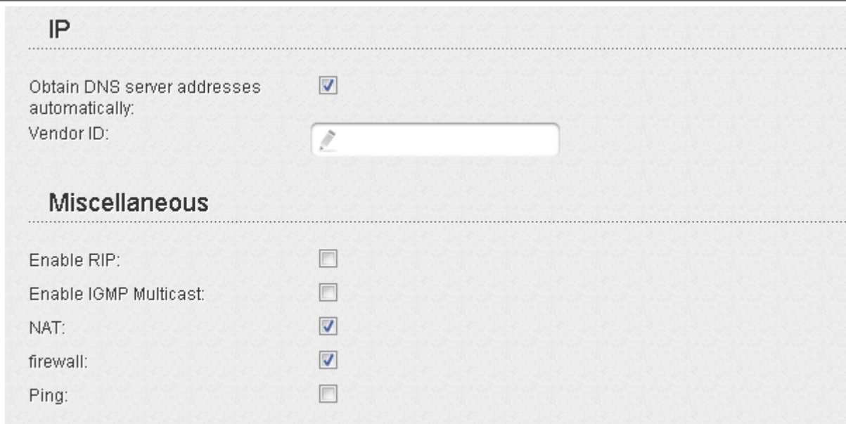
Figure 84. The page for creating a new connection. The IP and Miscellaneous sections.
