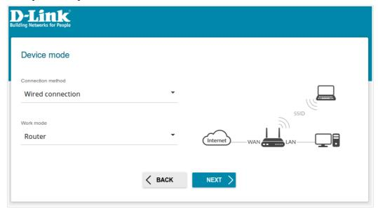
Figure 25. Selecting an operation mode. The Router mode.
