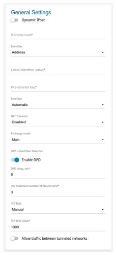
Figure 117. The page for adding an IPsec tunnel. The **General Settings** section.
