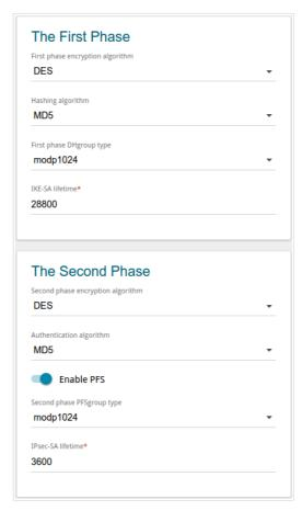
Figure 118. The page for adding an IPsec tunnel. The First Phase / The Second Phase sections.
