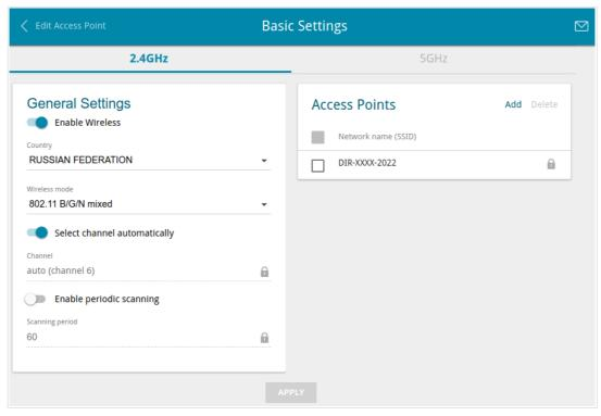
Figure 81. Basic settings of the wireless LAN in the 2.4GHz band.
