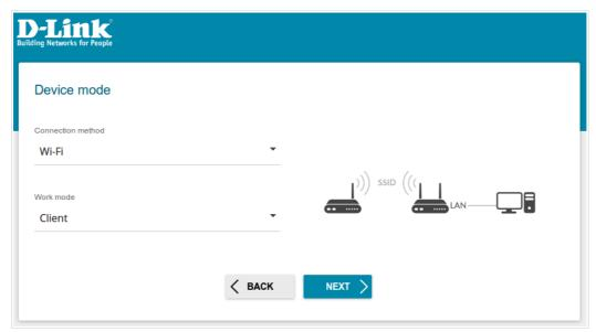
Figure 29. Selecting an operation mode. The Client mode.
