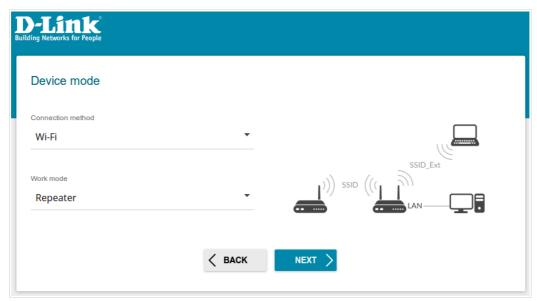
Figure 28. Selecting an operation mode. The Repeater mode.
