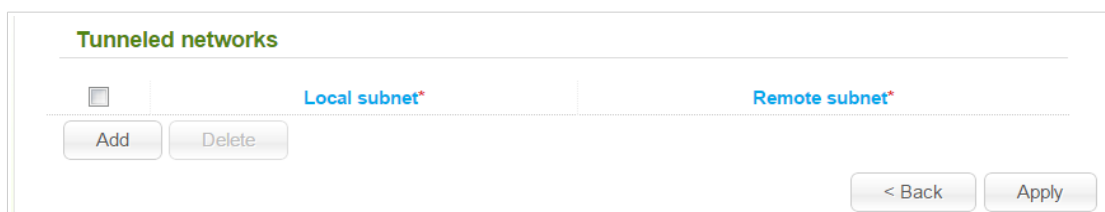
Figure 147. The page for adding an IPsec tunnel.
