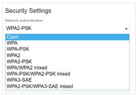
Figure 101. Network authentication types supported by the router.
