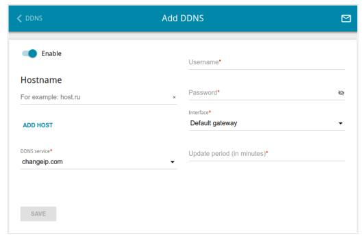
Figure 121. The page for adding a DDNS service.
