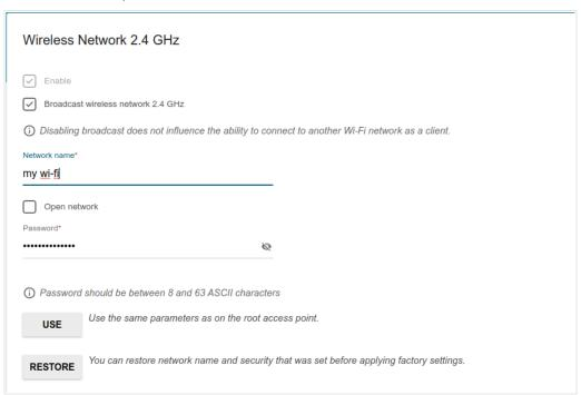
Figure 49. The page for configuring the wireless network.
