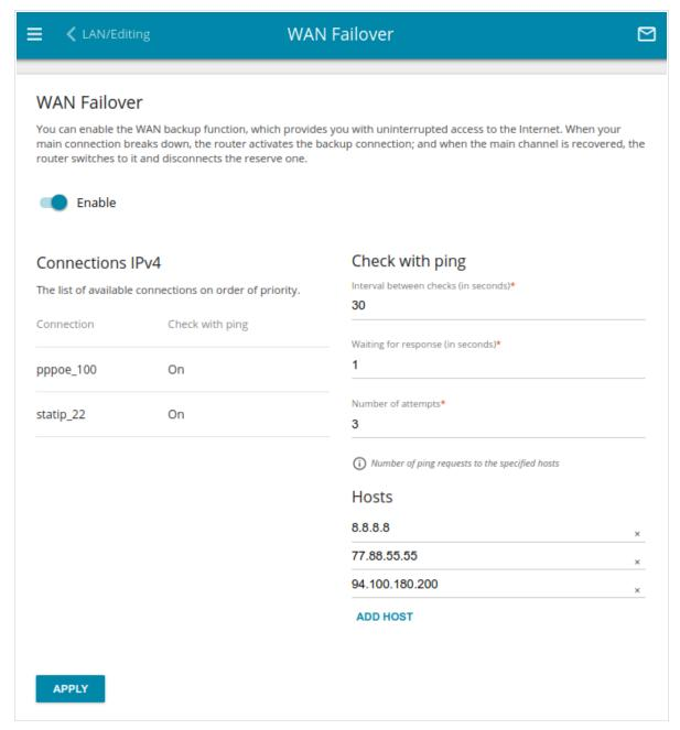
Figure 97. The Connections Setup / WAN Failover page.
