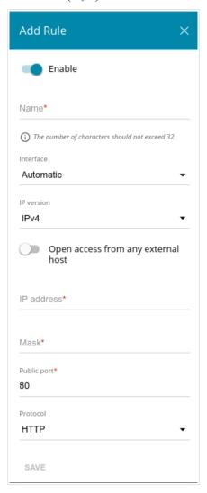
Figure 150. The window for adding a rule for remote management.
