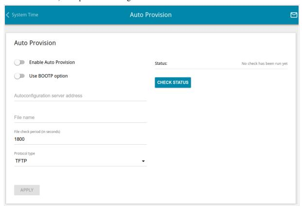
Figure 164. The page for configuring the Auto Provision function.
