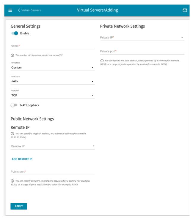
Figure 143. The page for adding a virtual server.
