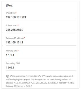
Figure 70. The page for creating a new Static IPv4 connection. The IPv4 section.
