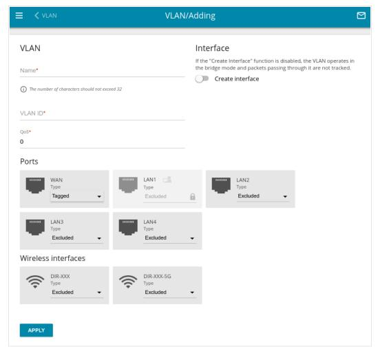
Figure 118. The page for adding a VLAN.
