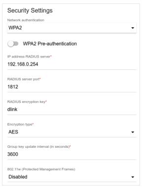
Figure 104. The WPA2 value is selected from the Network authentication drop-down list.
