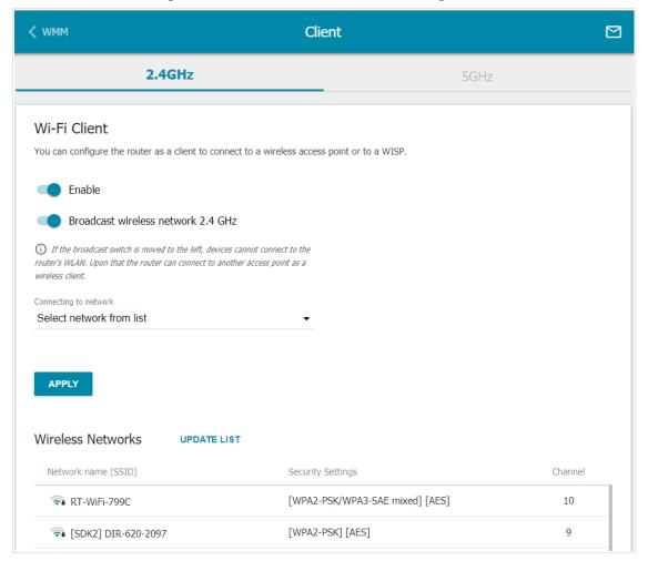
Figure 109. The page for configuring the client mode.
