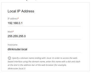
Figure 87. Configuring the local interface. The IPv4 tab. The Local IP Address section.
