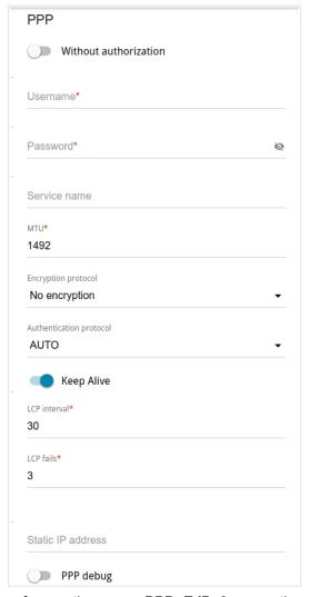
Figure 84. The page for creating a new **PPPoE IPv6** connection. The **PPP** section.
