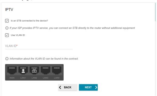
Figure 51. The page for selecting a LAN port to connect an IPTV set-top box.
