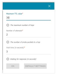
Figure 161. The **System / Traceroute** page. The additional settings window.
