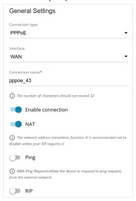
Figure 74. The page for creating a new **PPPoE** connection. The **General Settings** section.
