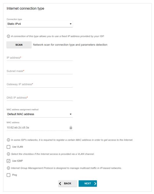
Figure 43. The page for configuring Static IPv4 WAN connection.
