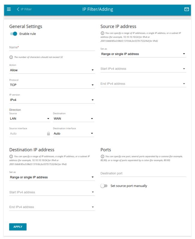
Figure 141. The page for adding a rule for IP filtering.
