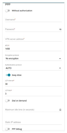
Figure 79. The page for creating a new PPTP connection. The PPP section.
