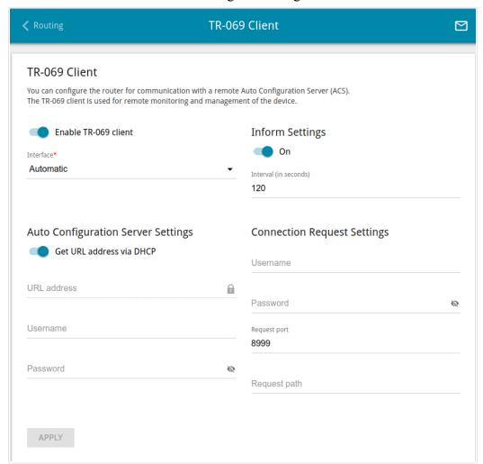
Figure 127. The page for configuring the TR-069 client.
