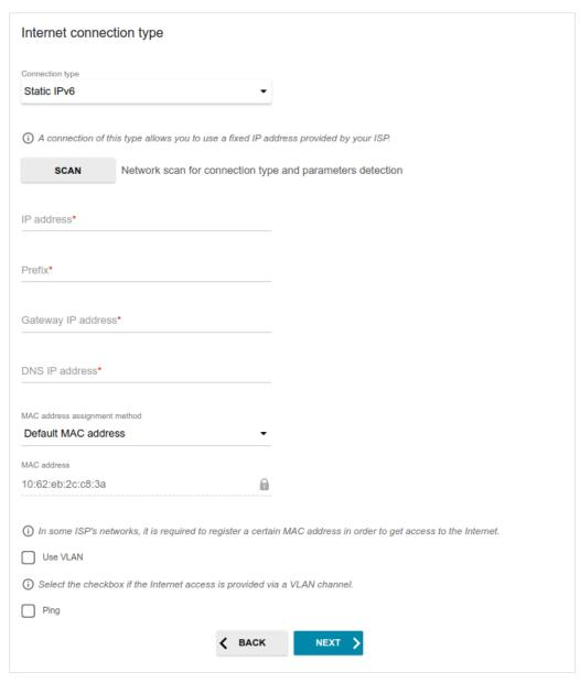
Figure 44. The page for configuring Static IPv6 WAN connection.
