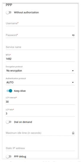
Figure 76. The page for creating a new **PPPoE** connection. The **PPP** section.
