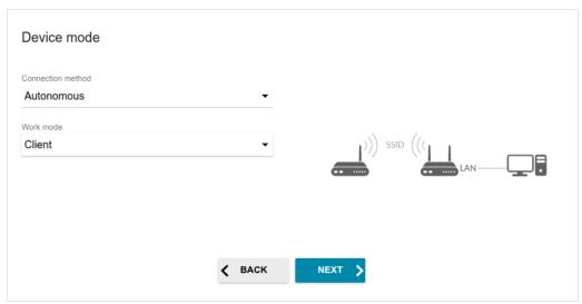
Figure 37. Selecting an operation mode. The Client mode.
