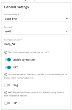
Figure 68. The page for creating a new Static IPv4 connection. The General Settings section.
