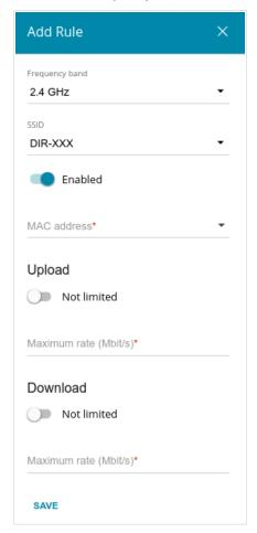
Figure 111. The window for setting up rate limit.
