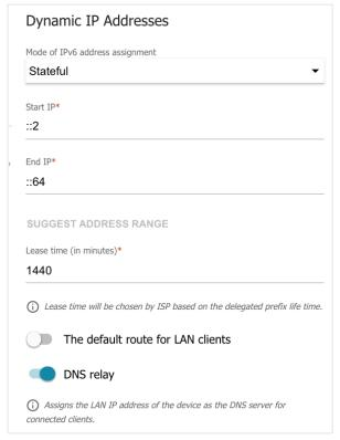
Figure 94. Configuring the local interface. The **IPv6** tab. The **Dynamic IP Addresses** section.
