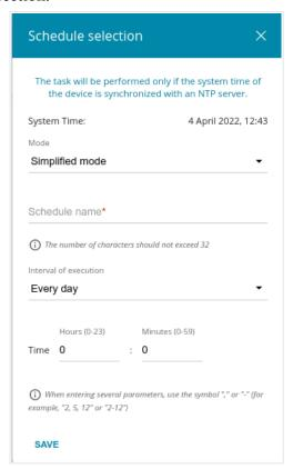
Figure 154. The window for configuring automatic reboot on a schedule.
