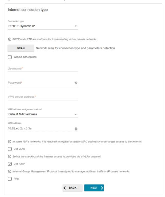
Figure 47. The page for configuring PPTP + Dynamic IP WAN connection.
