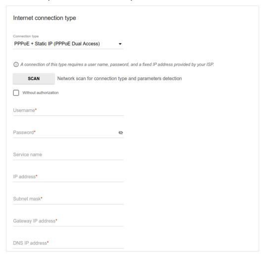
Figure 46. The page for configuring PPPoE + Static IP (PPPoE Dual Access) WAN connection.
