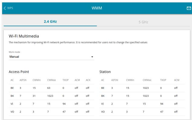
Figure 107. The page for configuring the WMM function.
