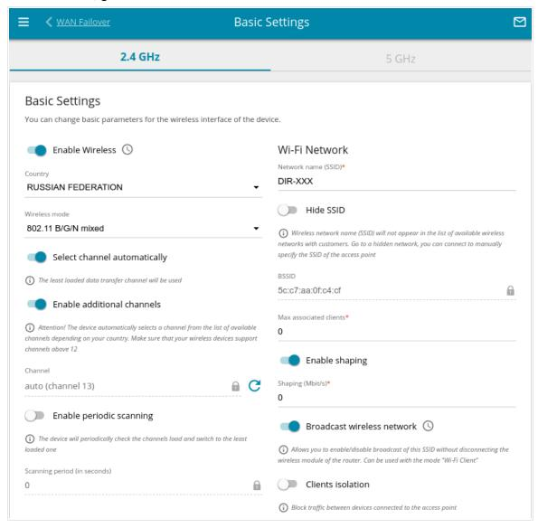
Figure 99. Basic settings of the wireless LAN in the 2.4GHz band.
