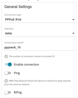
Figure 82. The page for creating a new PPPoE IPv6 connection. The General Settings section.
