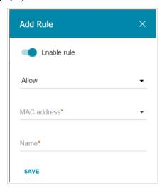
Figure 146. The window for adding a rule for the MAC filter.
