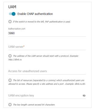
Figure 139. The page for adding an authorization server. The UAM section.
