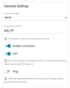
Figure 78. The page for creating a new **PPTP** connection. The **General Settings** section.
