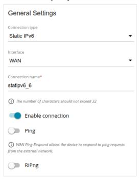
Figure 71. The page for creating a new Static IPv6 connection. The General Settings section.
