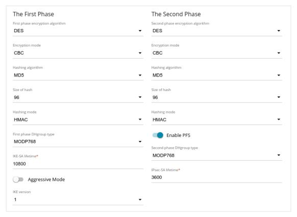
Figure 133. The page for adding an IPsec tunnel. The First Phase / The Second Phase sections.
