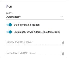
Figure 86. The page for creating a new PPPoE Pv6 connection. The IPv6 section.
