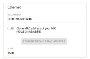
Figure 75. The page for creating a new **PPPoE** connection. The **Ethernet** section.
