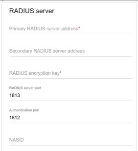
Figure 137. The page for adding an authorization server. The RADIUS server section.
