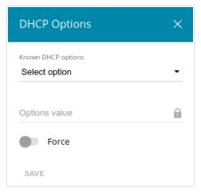
Figure 90. Configuring the local interface. The **IPv4** tab. The window for configuring a DHCP option. In the opened window, you can specify the following parameters:
