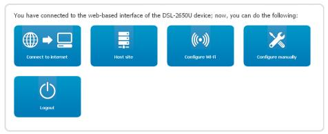
On the page, you can proceed to the Wizards (use the **Connect to internet**, **Host site**, and **Configure Wi-Fi** buttons) or switch to the standard webbased interface of the router by clicking the **Configure manually** button. After clicking the button, the system statistics page opens. The page displays general information on the router and its software, and data on the DSL connection state.
