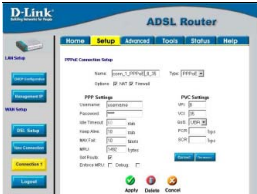
Figure 3-6. Setup – Configure Connection 1 for PPPoE
