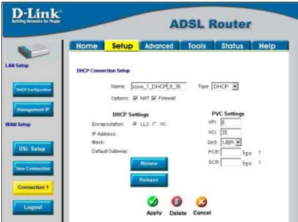
Figure 3-9. Setup – Configure Connection 1 for DHCP service for the WAN
