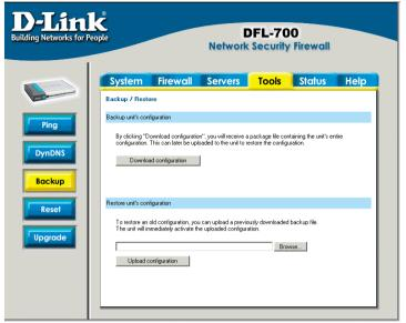
can restore the firewall's configuration file with the one stored on disc.
