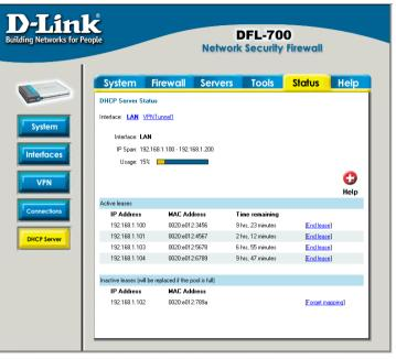
**Inactive leases** are leases that are not currently in use but have been used by a computer before, that computer will get that lease the next time it is on the network. If there is no free IP in the pool these IP's will be used for new computers.
