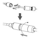
Screw the back part of the waterproof connector clockwise until there is a tight seal around the Ethernet cable.
