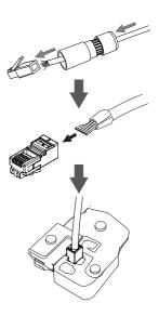
Connect the RJ-45 plug into the Ethernet connector, then screw the waterproof connector to the Ethernet connector by turning it about a half-turn clockwise.
