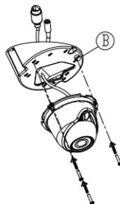
Remove the inner cover and adjust the angle and rotation of the camera as desired, then put the inner cover back in place.
