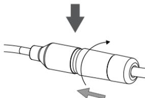
Turn the back part of the waterproof connector clockwise until there is a tight seal around the Ethernet cable.
