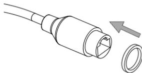
Thread bare Ethernet cable through the waterproof connector as shown, then crimp an RJ-45 plug onto the cable.
