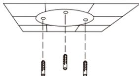
**If you are running the camera cables through the wall or ceiling**, drill a hole in the center and pull the cables through the hole. If not, then guide the camera cables through the cable channel on the base after mounting to the wall or ceiling.
