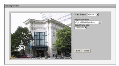
Once finished with the setting in the Viewing Window, click **Save** to enable the settings and click **Close** to exit the window. The selected Output Frame Size will immediately be applied to the Frame size of video stream. You can then go back to the Live Video to test the new settings.
