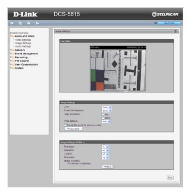
Brightness: Adjust the image brightness level, which ranges from -5 to +5
