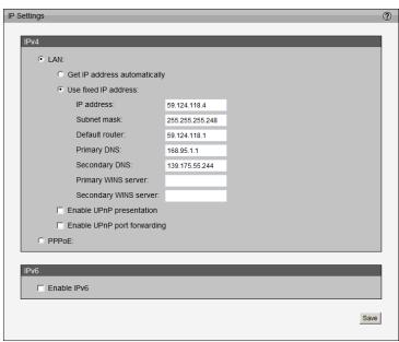
**Secondary WINS Server:** The secondary WINS server that maintains the database of computer name and IP address.
