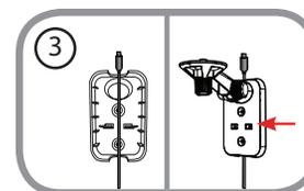
4. Fasten the mounting bracket to the wall using the screws provided.
