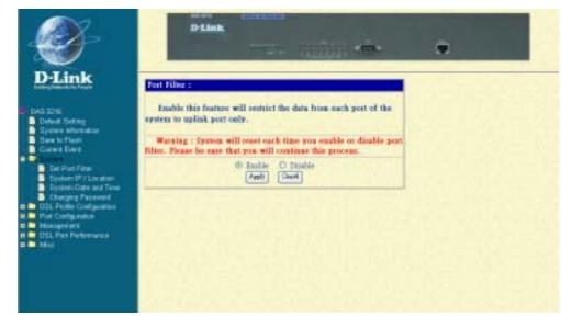
2. Click on **Enabled** button to allow each ADSL port to communicate back and forth with the uplink Ethernet port only.
