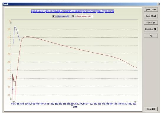
Figure 11-120 Graph of Loop Monitoring - Quiet Line Noise PSD
