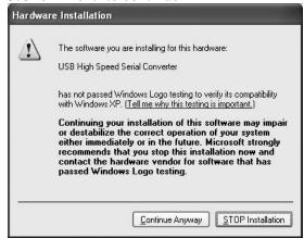
5. Click "Continue anyway" to proceed to install the "USB High Speed Serial Converter".
