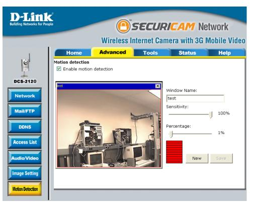
**Percentage:** Adjusting the percentage allows you to set a requirement on how much of the motion window must be filled by movement. Example: If you set this to 50%, then the selected window must be half filled by a moving object before it triggers motion detection.
