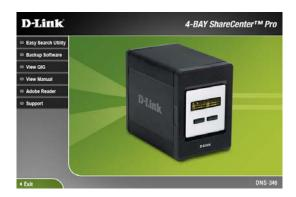
1. Click Easy Search Utility. The Easy Search Utility will load and detect any DNS-346 devices that are on the local network. If the DNS-346 you are working with does not show up in the device list, click Refresh.
