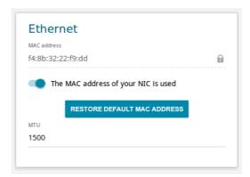
Figure 67. The page for creating a new **Static IPv6** connection. The **Ethernet** section.
