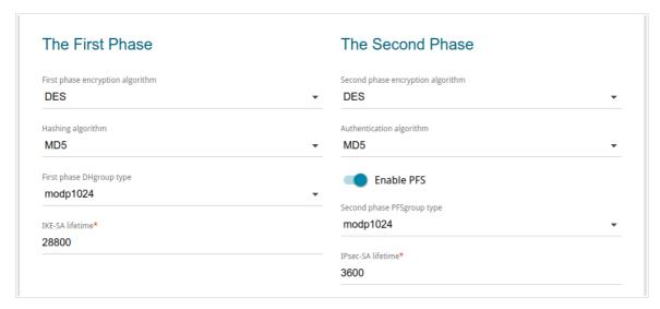
Figure 154. The page for adding an IPsec tunnel. The First Phase / The Second Phase sections.
