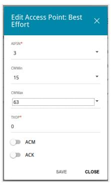
Figure 105. The window for changing parameters of the WMM function.
