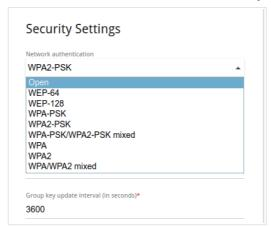
Figure 98. Network authentication types supported by the router.
