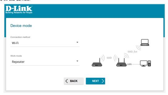
Figure 30. Selecting an operation mode. The Repeater mode.
