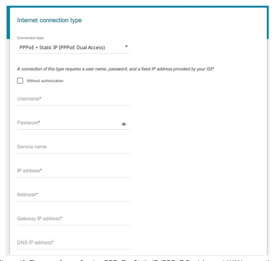
Figure 40. The page for configuring PPPoE + Static IP (PPPoE Dual Access) WAN connection.
