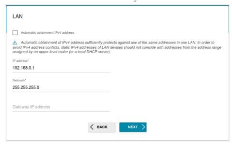
Figure 34. The page for changing the LAN IPv4 address.
