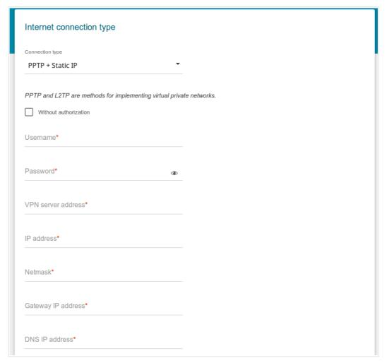
Figure 42. The page for configuring PPTP + Static IP WAN connection.
