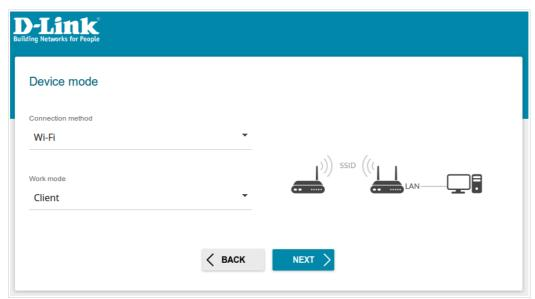
Figure 31. Selecting an operation mode. The Client mode.
