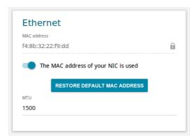
Figure 62. The page for creating a new **Static IPv4** connection. The **Ethernet** section.
