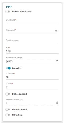
Figure 79. The page for creating a new **PPPoE IPv6** connection. The **PPP** section.
