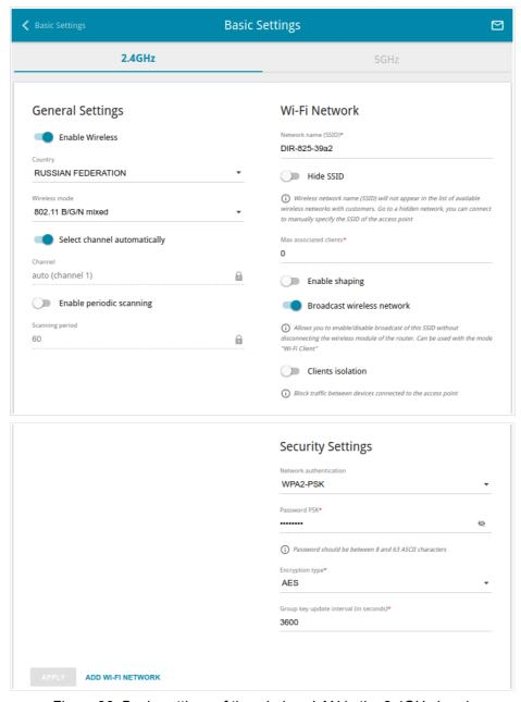
Figure 96. Basic settings of the wireless LAN in the 2.4GHz band.
