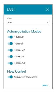
Figure 138. The window for changing the settings of the router's port.
