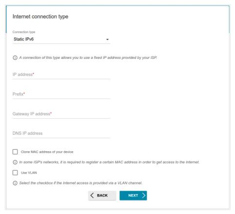
Figure 38. The page for configuring Static IPv6 WAN connection.
