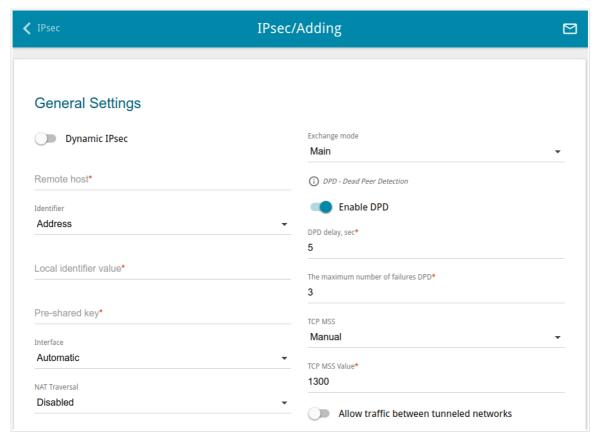
Figure 153. The page for adding an IPsec tunnel. The General Settings section.
