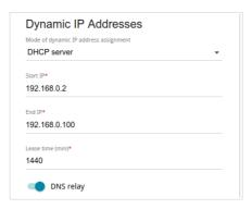
Figure 91. Configuring the local interface. The IPv4 tab. The Dynamic IP Addresses section.
