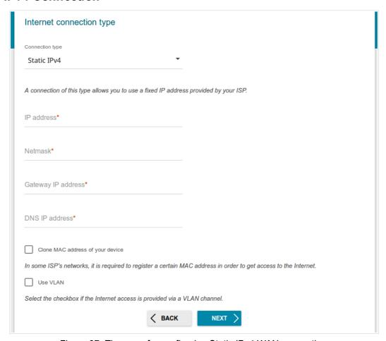
Figure 37. The page for configuring Static IPv4 WAN connection.
