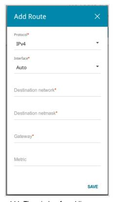
Figure 144. The window for adding a new route.
