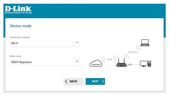
Figure 28. Selecting an operation mode. The WISP Repeater mode.
