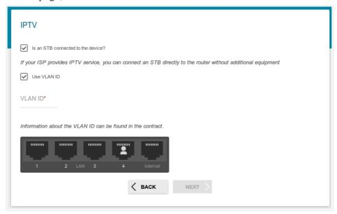
Figure 45. The page for selecting a LAN port to connect an IPTV set-top box.
