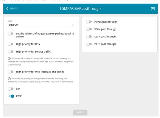
Figure 151. The Advanced / IGMP/ALG/Passthrough page.
