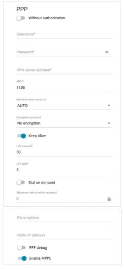
Figure 75. The page for creating a new **PPTP** connection. The **PPP** section.
