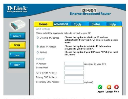
Choose Static IP Address if all WAN IP information is provided to you by your ISP. You will need to enter in the IP address, subnet mask, gateway address, and DNS address(es) provided to you by your ISP. Each IP address entered in the fields must be in the appropriate IP form, which are four IP octets separated by a dot (x.x.x.x.x). The Router will not accept the IP address if it is not in this format.
