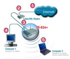
Please remember that **D-Link AirPlus** wireless devices are pre-configured to connect together, right out of the box, with the default settings.
