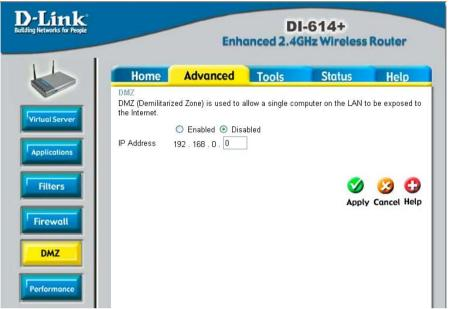
If you have a client PC that cannot run Internet applications properly from behind the DI-614+, then you can set the client up to unrestricted Internet access. It allows a computer to be exposed to the Internet. This feature is useful for gaming purposes. Enter the IP address of the internal computer that will be the DMZ host. Adding a client to the DMZ (Demilitarized Zone) may expose your local network to a variety of security risks, so only use this option as a last resort.
