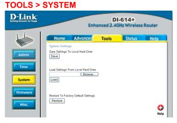
local hard drive and locate the system file to be used. You may also reset the Broadband Router back to factory settings by clicking on **Restore**.
