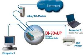
With the DI-704UP you can share Internet access and resources such as printers in your home or office. Connect up to four computers and a printer with the DI-704UP's USB printer port.
