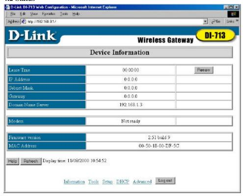
This option provides observation of the DI-713's configuration status. If the WAN port is assigned a dynamic IP address, a "Renew" or "Release" button may appear. You can click this button to manually renew or release the IP. This screen also provides the Firmware Version and MAC Address information. Pressing the Refresh button will update the Device Information screen to show the current status.
