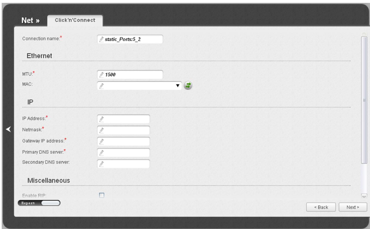
Figure 31. Configuring Static IP WAN connection. The expert settings mode. The Ethernet section.
