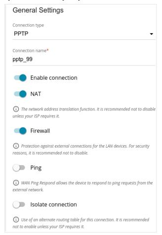
Figure 72. The page for creating a new **PPTP** connection. The **General Settings** section.
