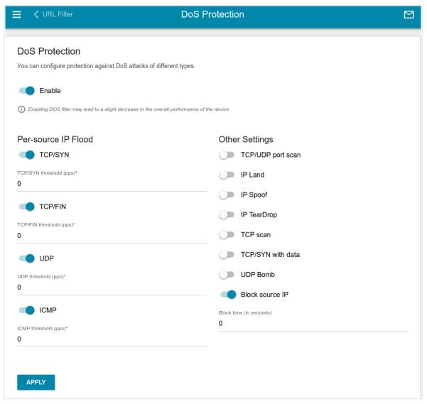
Figure 133. The Firewall / DoS Protection page.
