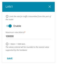
Figure 113. The window for setting up rate limit.
