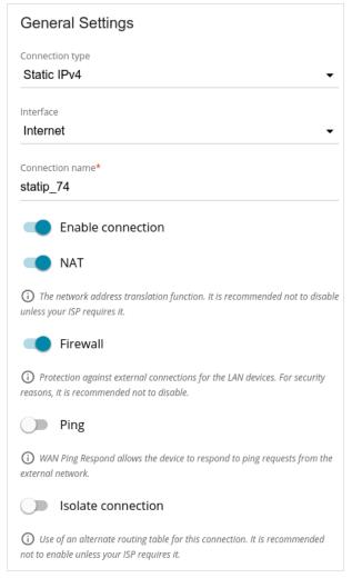
Figure 63. The page for creating a new Static IPv4 connection. The General Settings section.
