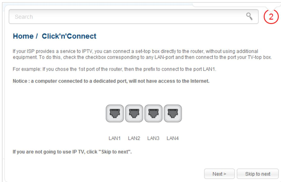
Figure 75. Selecting a LAN port to connect an IPTV set-top box.
