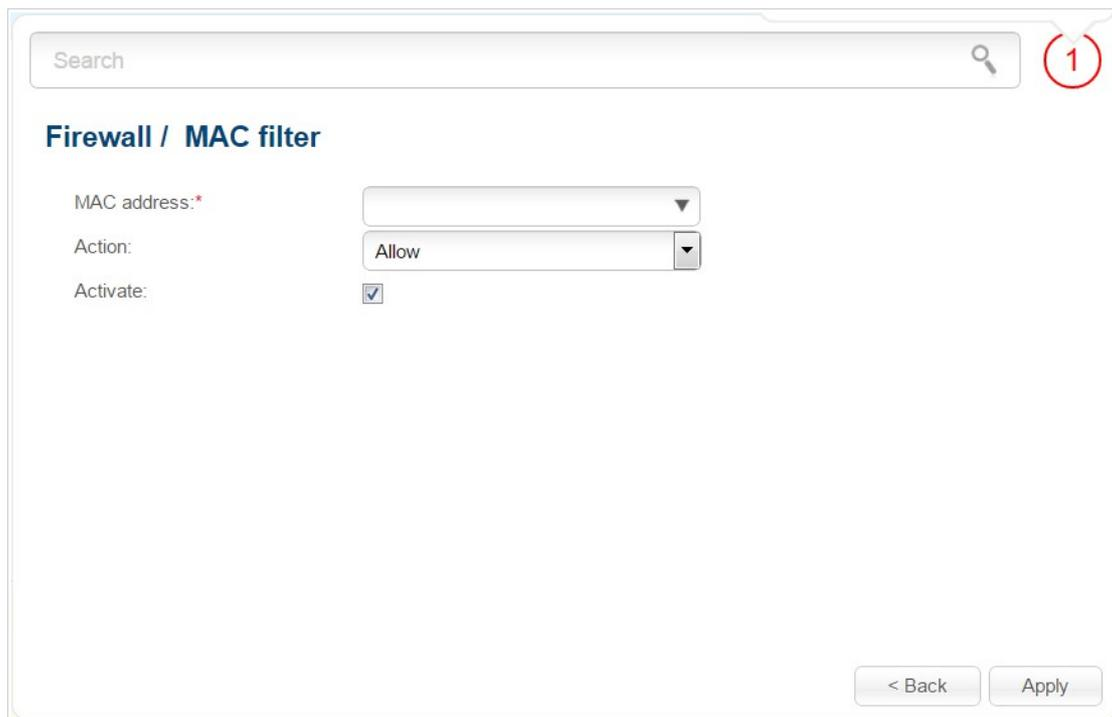
Figure 158. The page for adding a rule for the MAC filter.
