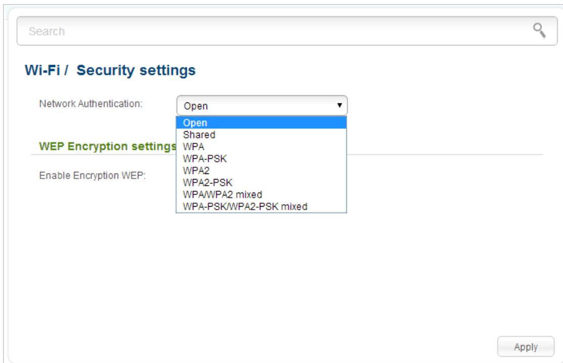
Figure 130. Network authentication types supported by the router.
