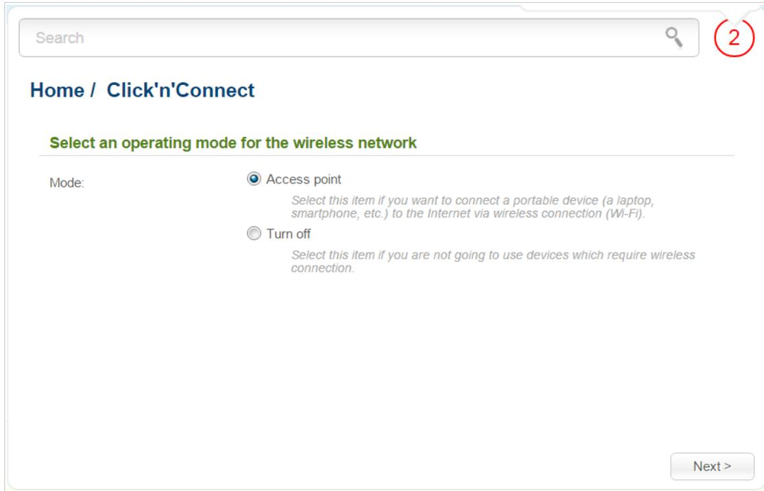
Figure 72. Selecting the operating mode for the wireless network.
