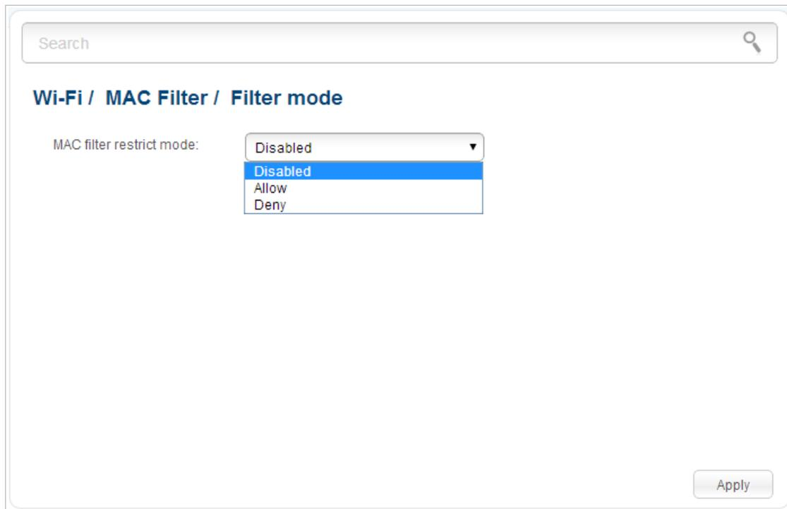
Figure 134. The page for configuring the MAC filter for the wireless network.
