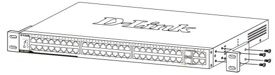
Figure 2 - 2. Fasten mounting brackets to Switch
