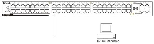
Figure 3-1. Switch connected to an end node
