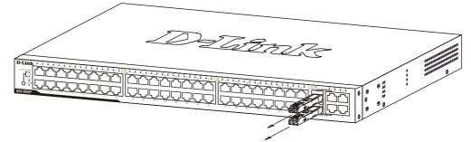
Figure 1-3. Inserting the fiber-optic transceivers into the DES-3028/28P/52/52P Switch
