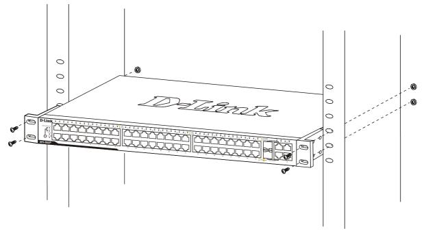
Figure 2 - 3. Installing Switch in a rack
