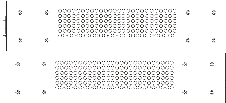
Figure 1-40. Side panels of the DES-3200-10
