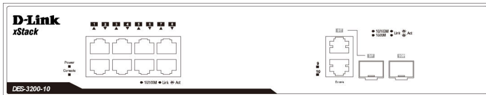
Figure 1-1. Front Panel of the DES-3200-10
