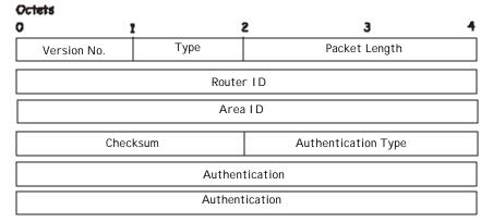
Figure 9 - 16. OSPF Packet Header Format
