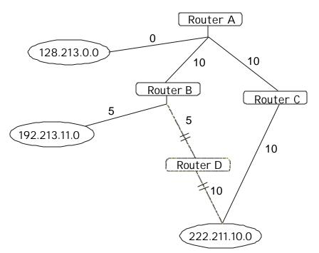
Figure 9 - 14. Constructing a Shortest Path Tree
