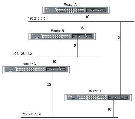
Figure 9 - 13. Constructing a Shortest Path Tree
