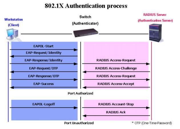
Figure 7 - 58. The 802.1x Authentication Process
