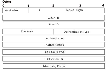
Figure 9 - 19. Link-State Request Packet
