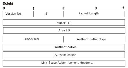
Figure 9 - 21. Link State Acknowledge Packet
