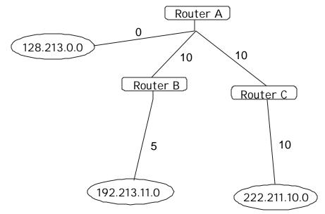
Figure 9 - 15. Constructing a Shortest Path Tree – Completed
