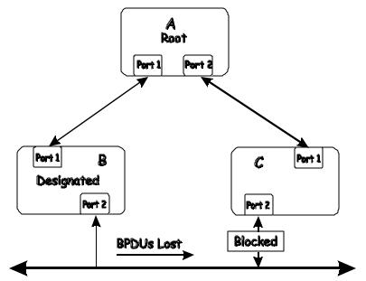
In this example, port 2 on B can receive but not transmit packets. Port 2 on C should be in the blocking state, but since it can no longer receive BPDUs from port 2 on B, it will transition to the forwarding state. If the failure exists at boot, STP will not converge and rebooting the bridges will have no effect. (Note: Rebooting would help temporarily in the previous example).
