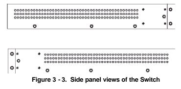
The system fans are used to dissipate heat. The sides of the system also provide heat vents to serve the same purpose. Do not block these openings, and leave at least 6 inches of space at the rear and sides of the switch for proper ventilation. Be reminded that without proper heat dissipation and air circulation, system components might overheat, which could lead to system failure.
