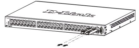
Figure 3 - 4. Mini-GBIC modules plug-in to the Switch
