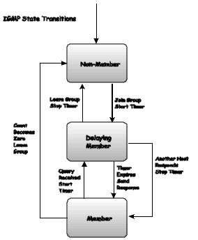
Figure 9 - 42. IGMP State Transitions
