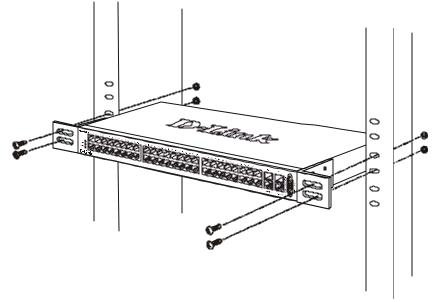
Figure 2 - 3. Installing the switch on an equipment rack
