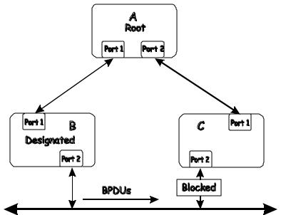
In this example, B has been elected as the designated bridge and port 2 on C is in the blocking state. The election of B as the designated bridge is determined by the exchange of BPDUs between B and C. B had a better BPDU than C. B continues sending BPDUs advertising its superiority over the other bridges on this LAN. Should C fail to receive these BPDUs for longer than the MAX AGE (default of 20 seconds), it could start to transition its port 2 from the blocking state to the forwarding state.
