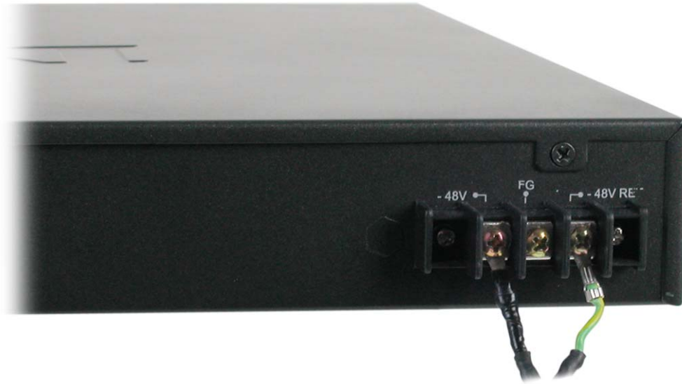
Figure 2 - 4. Power connections attached to contacts after assembly
