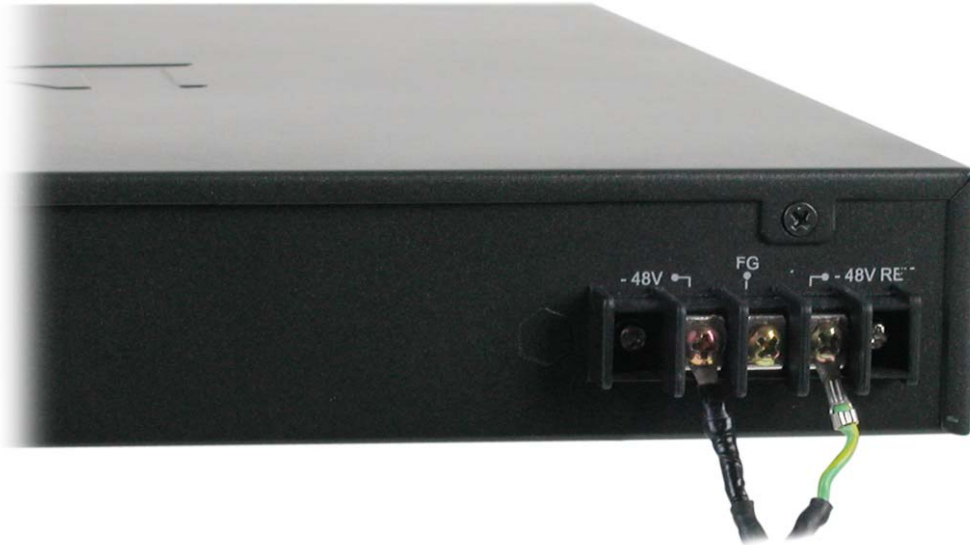
Figure 2 - 4. Power connections attached to contacts after assembly
