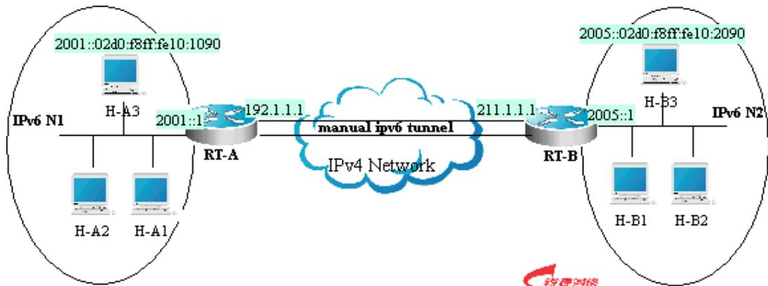
As shown in the above figure, IPv6 networks N1 and N2 are isolated by the IPv4 network. Now, the two networks are interconnected by configuring a manual tunnel. For example, the H-A3 host in N1 can access the H-B3 host in N2.
