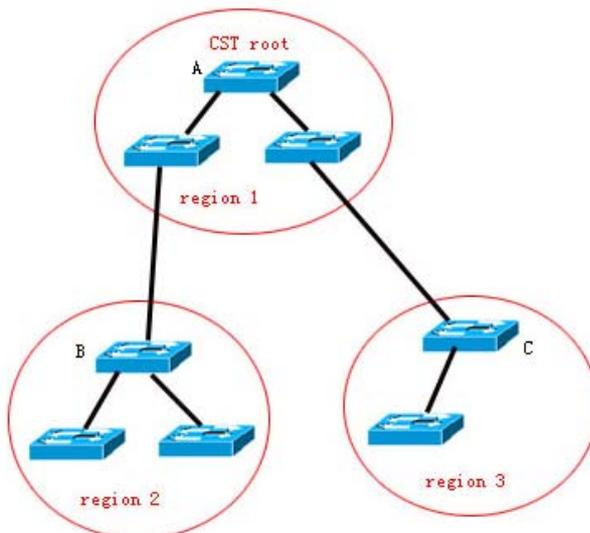
The CIST regional root needs not to be the switch with the smallest bridge ID within this region, which means the switch with the minimum root path cost to the CST root within this region.
