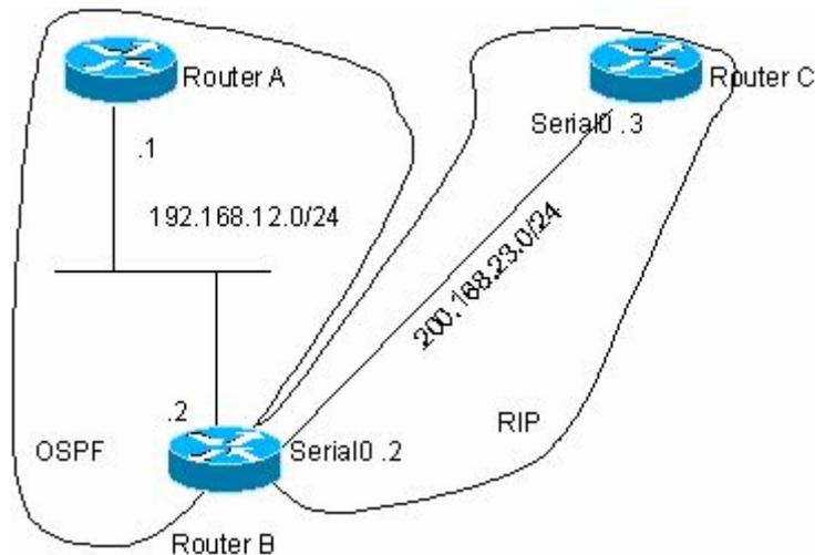
The OSPF only redistributes the routes in the RIP routing area and the route type is Type-1. The RIP only redistributes the 192.168.10.0/24 route in the OSPF routing area and its metric is 3.
