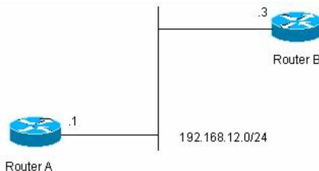
Router A must send RIP packets with the authentication key of keya and can receive the RIP packets whose authentication keys are keya and keyb. Router B sends the RIP packets with the authentication key of keyb and can receive the RIP packets of the authentication keys of keya and keyb.
