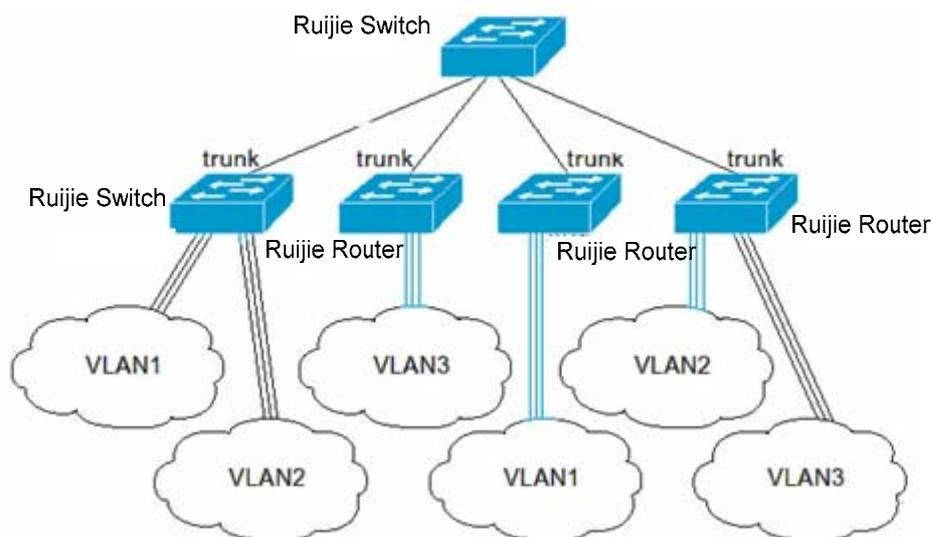
You can set one common Ethernet port or one Aggregate Port to be a Trunk port (For the details of Aggregate Port, see Configuring Aggregate Port).
