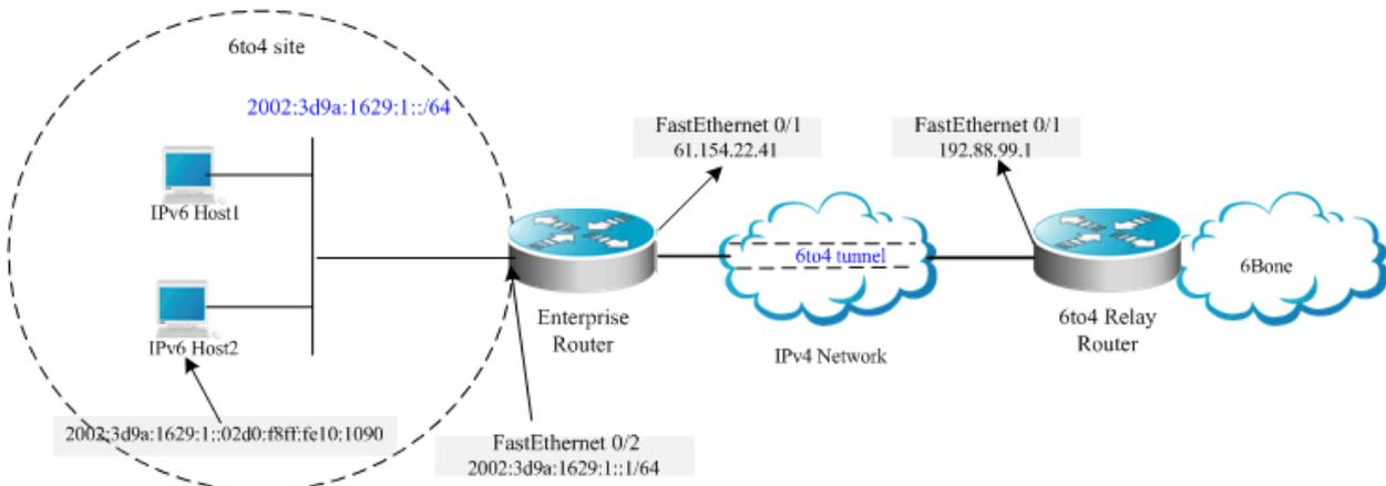
As shown in the above figure, an IPv6 network (6to4 site) uses a 6to4 tunnel to access the IPv6 backbone network (6bone) via the 6to4 relay router.
