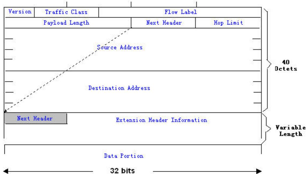
In the IPv4, all packet headers take 4 bytes as the unit. While in the IPv6, the packet header takes 8 bytes as the unit and the total length of the packet header is 40 bytes. IPv6 packet headers defines the following fields:
