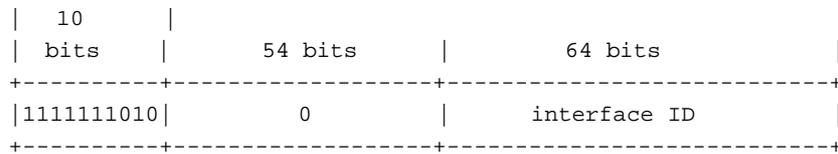
The link-level local address is used to number the host on the single network link. The address of former 10-bit identification for the prefix is the link-level local address. The router will not forward the message of the source address of the destination address with the link-level local address forever. The intermediate 54-bit of this address is 0. The latter 64 indicates the interface identifier, this part allows the single network to connect to up to  $2^{64}-1$  hosts.
