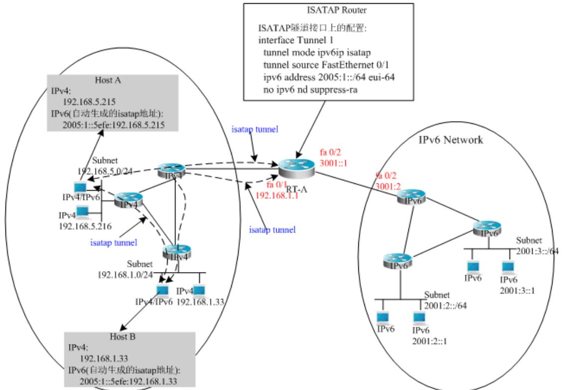
As shown in the above figure, it is one typical topology by use of an ISATAP tunnel. The ISATAP tunnel is used to communicate between isolated IPv4/IPv6 dual stack hosts inside the IPv4 site. The ISATAP router has the two following functions inside the ISATAP site:
