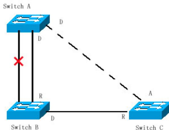
If the failure of the path between Switch B and Switch C occurs, the Switch C will switch the Alternate port to the Root port to generate the Figure R1w-3-4.
