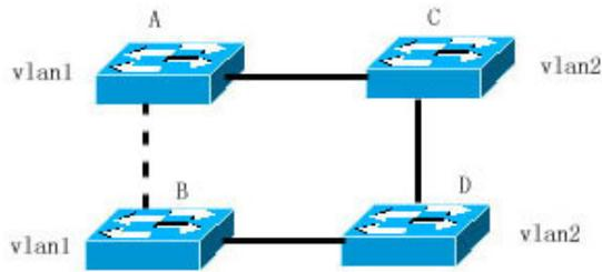
The MSTP is developed to address this problem for it can partition one or more vlans of the switch into an instance, so the switches with the same instance configuration form a region (MST region) to run separate spanning tree (this internal spanning-tree is referred to as the IST). The combination of the MST region is equivalent to a large switch, which executes the spanning tree algorithm with other MST region to obtain a common spanning tree, referred to as the common spanning tree (CST).
