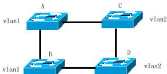
For some specified configuration, it will cause the DISCARDING of the path between the switch A and B (as Figure *mstp-2*). For the switch C and D don't include vlan1, it can't forward the data packet of vlan1, so the vlan1 of switch A fails to communicate with the vlan1 of switch B.
