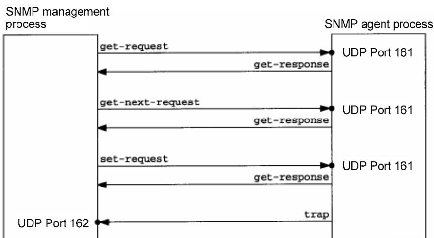
The first 3 operations from NMS to Agent and the response operation of the Agent are implemented on UDP port 161. The trap operation from Agent is implemented on UDP port 162.
