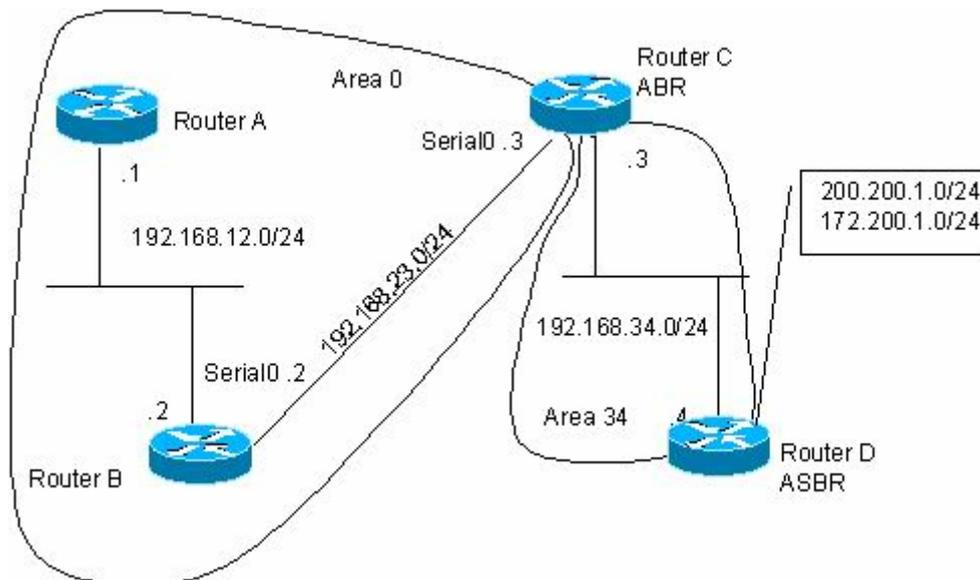
As shown in the diagram, routers A and B are within the area, while router C is an ABR, and router D is an ASBR. 200.200.1.0/24 and 172.200.1.0/24 are the networks outside the OSPF routing area. Configure various routers so that all OSPF routers can learn the external routes, which must carry the “34” tag and be Type-1.
