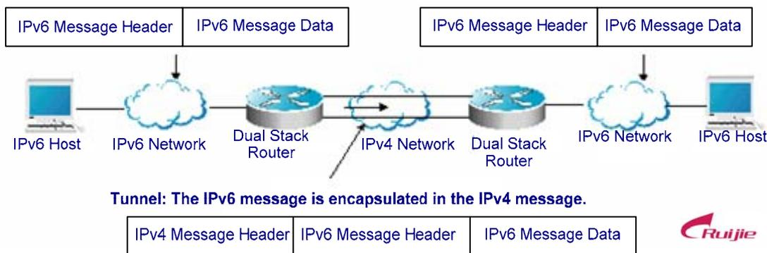
The features of various tunnels are respectively introduced below.
