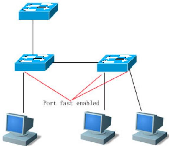
If the BPDU is received from the port with the Port Fast set, its Port Fast operational state is disabled. At this time, this port will execute the forwarding by normal STP algorithm.
