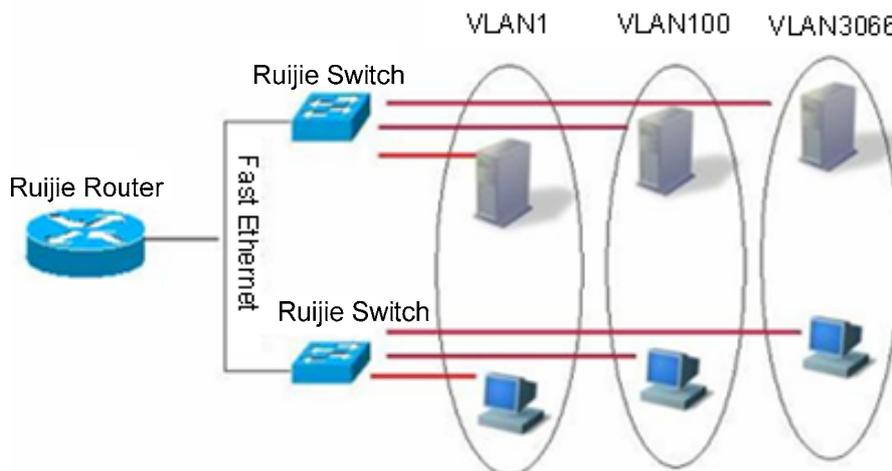
Same as a physical network, the VLAN is usually connected to an IP subnet. A typical example is that all the hosts in one IP subnet belong to the same VLAN. The communication between VLANs must go through a L3 device (router or L3 switch). Our L3 switch can perform IP routing between VLANs through the SVI (Switch Virtual Interfaces). For the configuration about the SVI, please see Interface Management Configuration and Configuring IP Unicast Routing Configuration.
