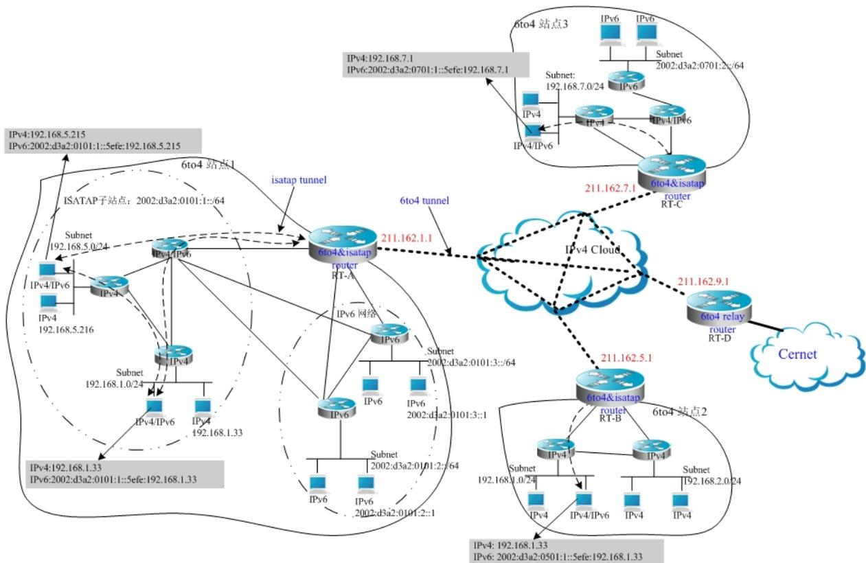
In the above figure, it is an instance about composite application of 6to4 tunnel and ISATAP tunnels. By use of the 6to4 tunnel technology, various 6to4 sites are interconnected and the 6to4 site accesses the Cernet network via the 6to4 relay router. At the same time, by use of the ISATAP tunnel technology inside the 6to4 site, the IPv6 hosts isolated by IPv4 inside the site perform IPv6 communication via the ISATAP tunnel.
