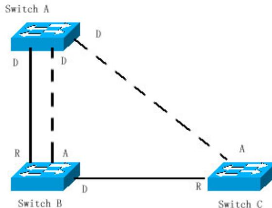
If the failure of the active path between Switch A and Switch B occurs, the alternate path will take action immediately to generate corresponding Figure R1w-3-3.
