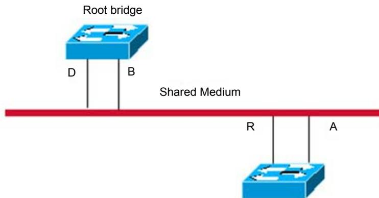
Each port takes three port states to indicate whether the data packet is forwarded, to control the topology of the whole spanning tree.
