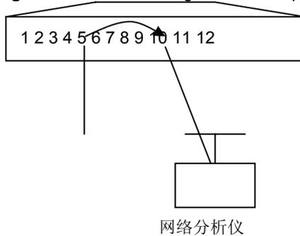
Through the SPAN, you can monitor all the frames incoming/outgoing the source port, including the route input frames.
