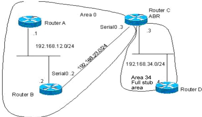
The requirement is that only the OSPF default route and the network routes of the local area can be seen in the routing table of Router D.
