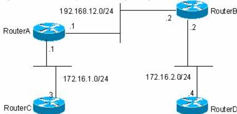
It is required to display routes of 172.16.2.0/24 on router C and display routes of 172.16.1.0/24 on router D by configuring RIP routing protocol to RIPv1.
