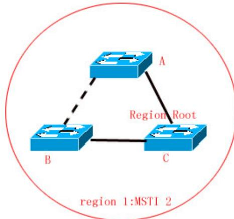
It should note that the MSTP protocol doesn't concern with which vlan the port is of, so users should configure corresponding path cost and priority for related port according to actual vlan configuration, to prevent the MSTP protocol from breaking the loop unexpected.
