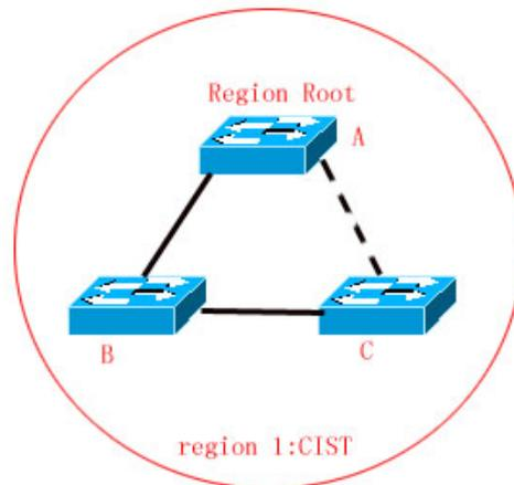
As is shown in Figure *mstp-4-2*, switch B with the highest priority is selected as the Region Root in the MSTI 1 (instance 1). Then, the path between switch B and C is DISCARDING according to other parameters. Hence, for the vlan group of the instance 1, only the path from switch A to B and switch B to C is available, which breaks the loop of the vlan group.
