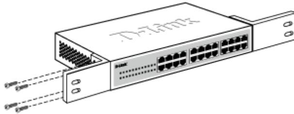
Figure 3-2 Attach the mounting brackets to the switch
