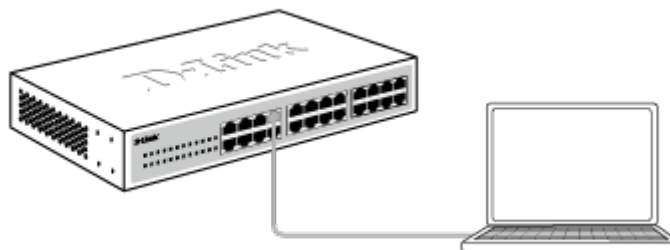
Figure 4-1 Connecting to a DGS-1100 MP/MPP Series switch
