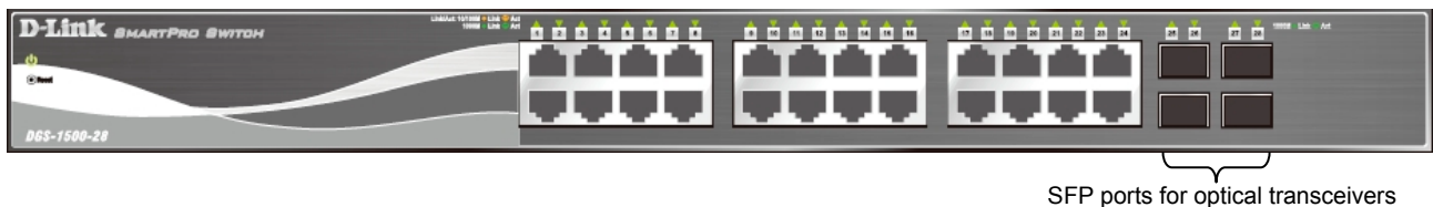
Figure 1.3 – DGS-1500-28 Front Panel
