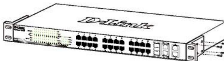
Figure 2.2 – Attach the mounting brackets to the Switch
