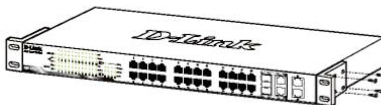
Figure 2.2 – Attach the mounting brackets to the Switch
