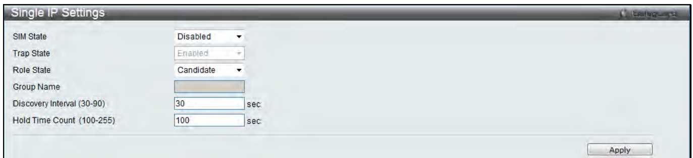
Figure 3-20 Single IP Settings window
