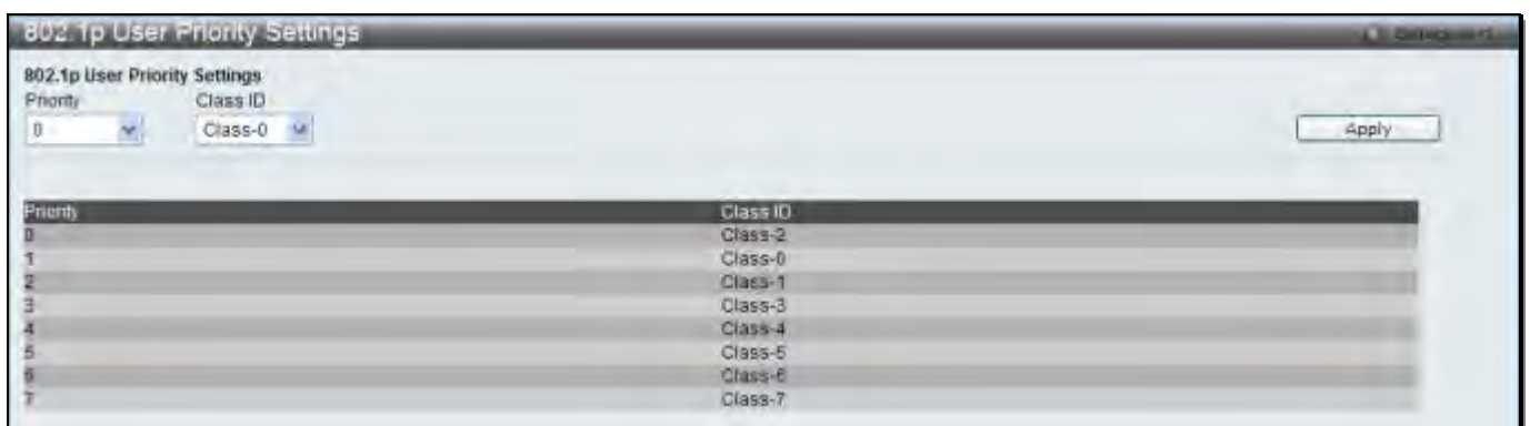
Figure 6-3 802.1p User Priority Settings window
