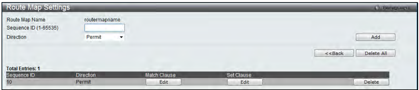
Figure 5-146 Route Map Settings - View Detail window
