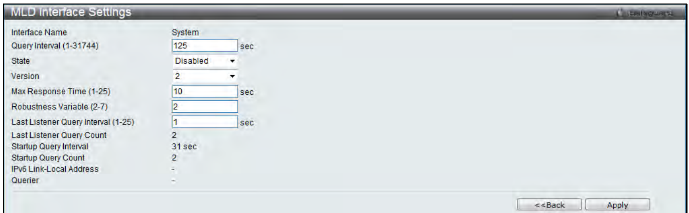
Figure 5-99 MLD Interface Settings –Edit window
