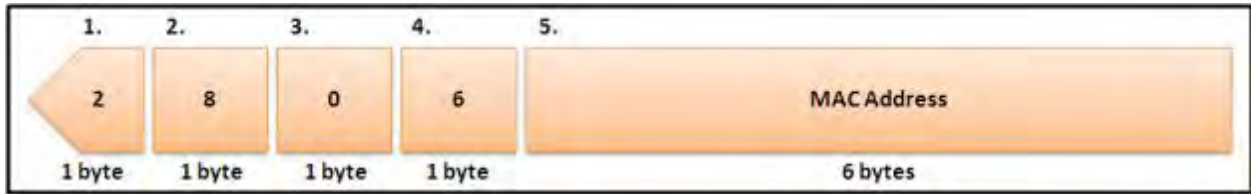
Figure 9-3 Remote ID Sub-option Format
