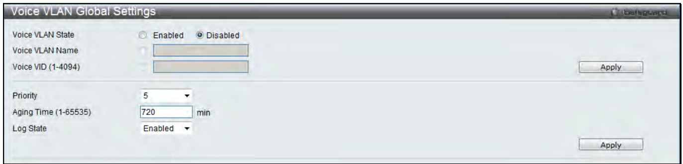
Figure 4-17 Voice VLAN Global Settings window
