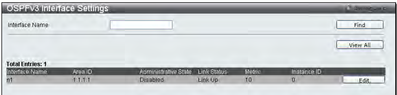
Figure 5-61 OSPFv3 Interface Settings window
