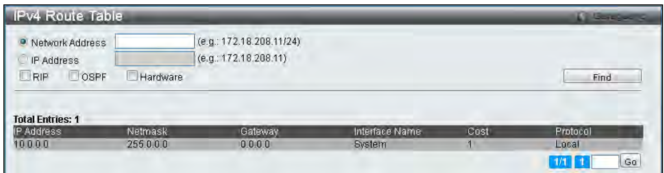
Figure 5-4 IPv4 Route Table window (RI Mode Only)
