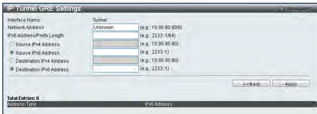
Figure 5-27 IP Tunnel GRE Settings (Edit) window
