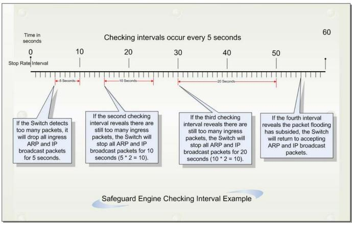
Figure 9-69 Safeguard Engine Checking Interval
