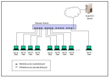
Figure 9-7 Example of Typical Port-based Configuration
