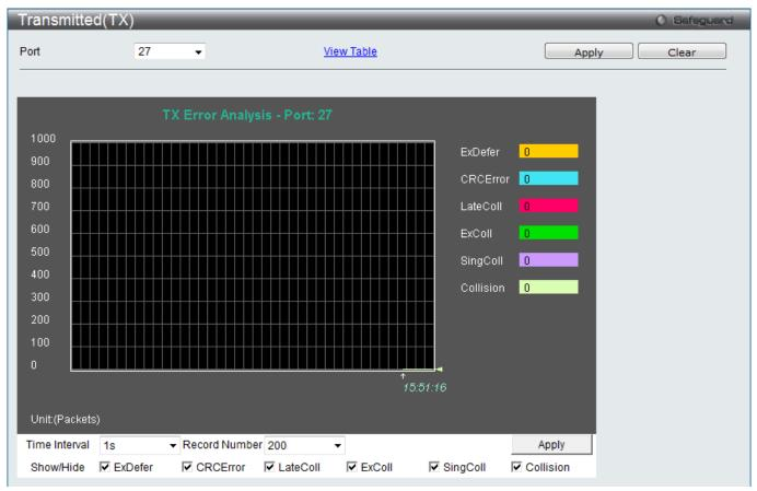
Figure 12-12 Transmitted (TX) window (for errors)
