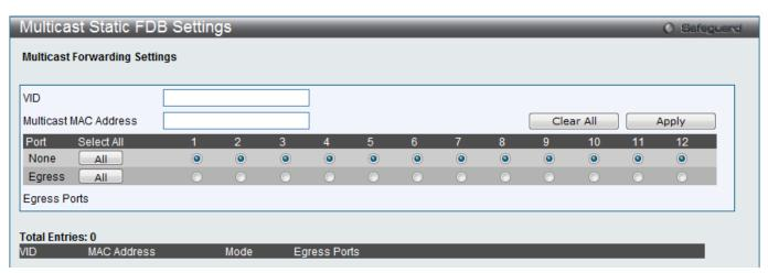
Figure 5-36 Multicast Static FDB Settings window
