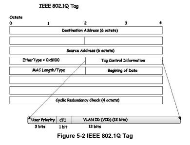
The EtherType and VLAN ID are inserted after the MAC source address, but before the original EtherType/Length or Logical Link Control. Because the packet is now a bit longer than it was originally, the Cyclic Redundancy Check (CRC) must be recalculated.
