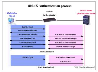
Figure 9-6 The 802.1X Authentication Process
