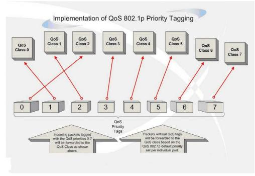
Figure 7-1 Mapping QoS on the Switch
