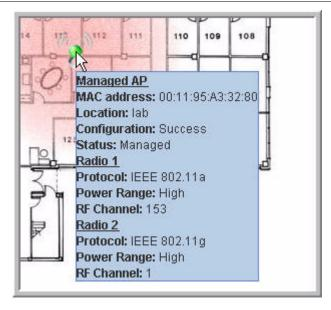
Figure 101. Tool Tip for Radio Managed AP Information
