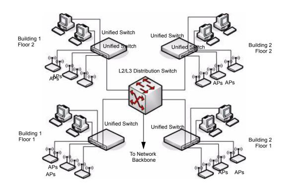
The four D-Link Unified Switches are in the same peer group. This allows wireless clients to roam between floors and between buildings without the need to re-authenticate. Additionally, each Unified Switch shares its list of managed APs and wireless clients with the switches in the peer group so that the APs and wireless clients are not reported as rogues (unknown).
