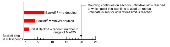
The random backoff used by the access point is a configurable parameter. To describe the random delay, a "Minimum Contention Window" (MinCW) and a "Maximum Contention Window" (MaxCW) is defined.
