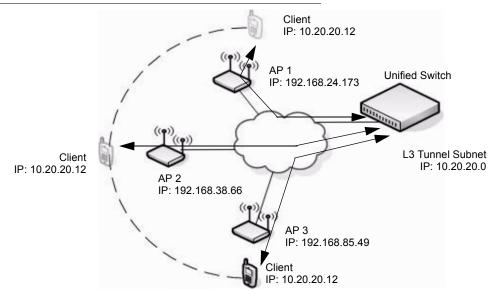
In the tunneling configuration, you can use ACL lists and QoS parameters to ensure that timesensitive traffic, such as VoIP, takes priority over other WLAN traffic.
