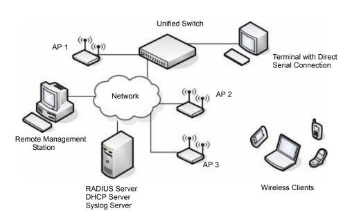
**NOTE:** The D-Link Unified Switch has a built-in DHCP server. If you do not already have a DHCP server on your network, you can configure the Unified Switch to assign network information to network hosts.
