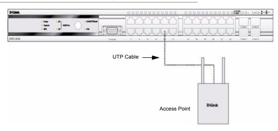
Figure 28. Switch and AP Connected Directly
