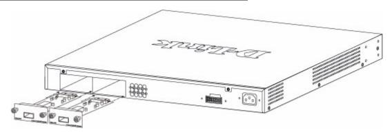
Now tighten the two screws at adjacent ends of the module into the available screw holes on the Switch. The upgraded Switch is now ready for use.
