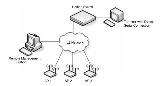
When the APs are on the same subnet and have the same SSID, wireless clients can seamlessly roam among the three APs with no interruption in network access. The client keeps the same IP address and does not need to re-authenticate when it moves into the broadcast area of a different AP. Configuration changes to the APs are managed by the switch simultaneously or on a per-AP basis.
