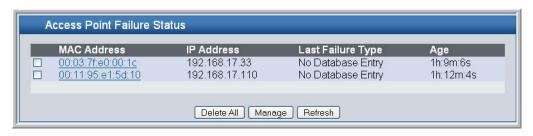
The AP authentication failure list shows information about APs that failed to establish communication with the D-Link Unified Switch. The AP can fail due to one of the following reasons:
