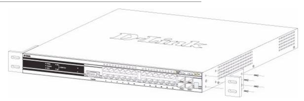
Figure 20. Fasten Mounting Brackets to Switch
