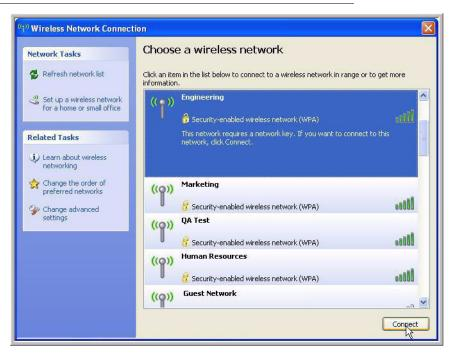
Although the wireless client finds five different wireless networks, these networks are all on the same access point. The D-Link Access Point looks like five separate access points to the wireless client.
