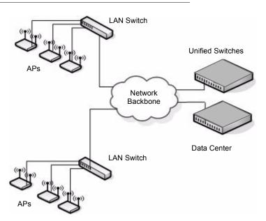
The data center topology is a good solution in networks where the goal is to add a wireless LAN to a network with minimal changes to the existing network. Traffic from wireless clients to the APs is either tunneled through the Unified Switch or tagged with a VLAN ID by the AP and handled accordingly. If the traffic is tagged, it might not pass through the Unified Switch.
