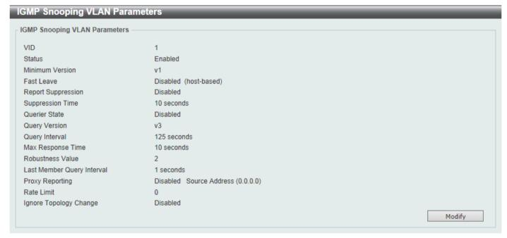
Figure 5-66 IGMP Snooping Settings (Show Detail) Window
