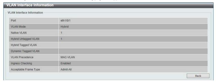
Figure 5-20 VLAN Interface (VLAN Detail) Window
