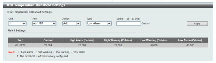
Figure 10-28 DDM Temperature Threshold Settings Window
