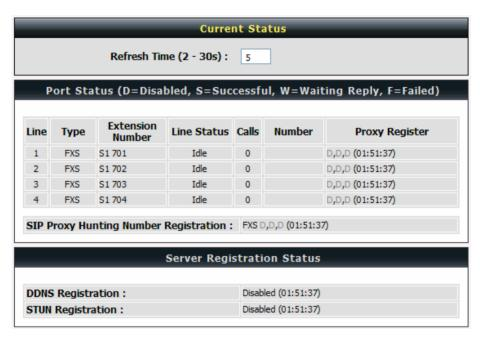
For Port Status, it includes if each port registers to Proxy successfully, the last dialed number, how many calls each port has made since the VoIP Gateway is start, etc.
