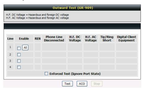
It allows operator to verify whether it is some problem on the cable between Phone Sets and DVG-5004S.
