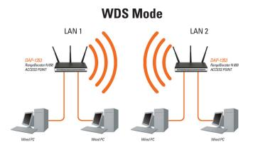
Connecting two separate LANs together through two DAP-1353 units (Wireless PCs cannot access the DAP-1353 units)
