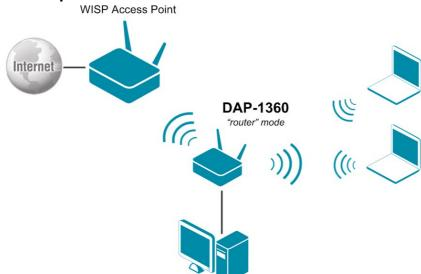
The DAP-1360 device in the "router" mode is connected to a WISP access point via wireless connection.
