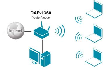
The DAP-1360 device in the "router" mode is connected to a private Ethernet line or to a cable or DSL modem. Computers connect to DAP-1360 via wireless or wired connection. It is necessary to specify the same encryption parameters and the channel of the wireless network for DAP-1360 and computers with Wi-Fi adapters. In addition, it is necessary to configure a WAN connection for DAP-1360.
