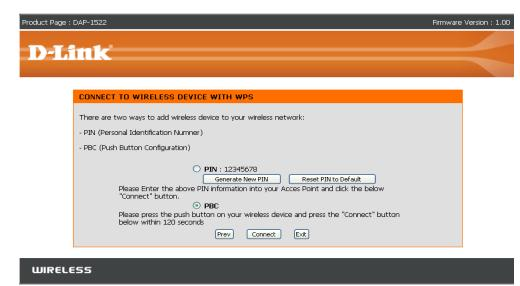
Press down the Push Button on the wireless device you are adding to your network to complete the setup.
