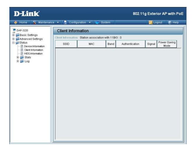
Client Information: This window displays the wireless client information for clients currently connected to the DAP-3220.
