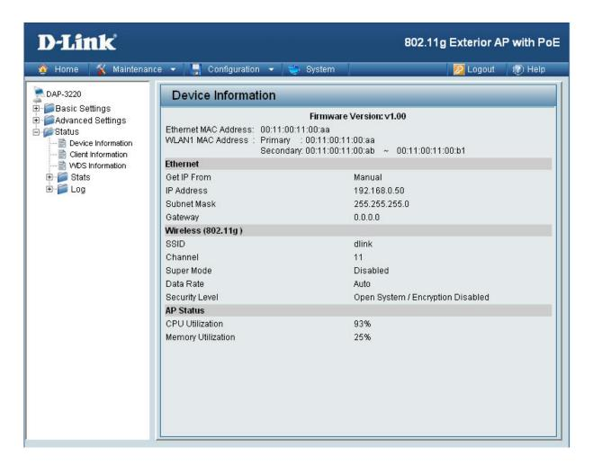
**Device Information:** This window displays the configuration settings of the DAP-3220, including the firmware version and the device's MAC address.
