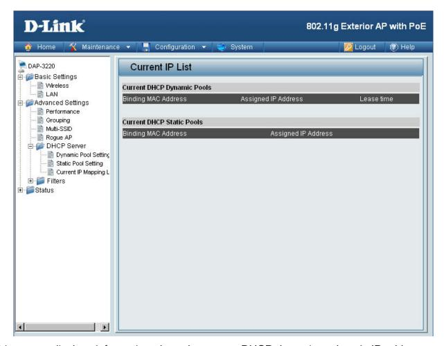
This screen displays information about the current DHCP dynamic and static IP address pools. This information is available when you enable the DHCP function of the DAP-3220 and assign dynamic and static IP address pools.
