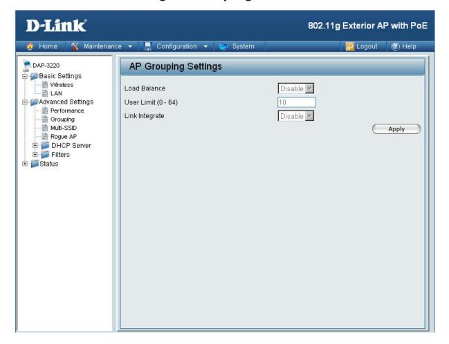
Load Balance: Allows you to balance and share the wireless network traffic and clients using multiple DAP-3220s. Select Enable or Disable.
