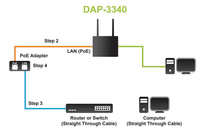
Connect one end of an Ethernet cable (included with your access point) to the LAN port on the DAP-3340 and the other end of the Ethernet cable to PoE power adapter.
