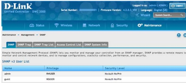
The screenshot shows the D-Link Unified Controller web interface. The top navigation bar includes Status, Wireless, Network, Security, and Maintenance. The Maintenance menu is expanded to show Management > SNMP. The SNMP menu is further expanded to show SNMP, SNMP Trap, SNMP Trap List, Access Control List, and SNMP System Info. The main content area displays the 'SNMP v3 User List' table.
