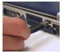
B. Firmly insert one end of the USB cable (larger plug) into your computer's USB Port.
