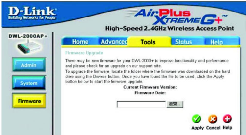
You can upgrade the firmware of the Access Point here. Make sure the firmware you want to use is on the local hard drive of the computer. Click on **Browse** to browse the local hard drive and locate the firmware to be used for the update. Please check the D-Link support site for firmware updates at <http://support.dlink.com>. You can download firmware upgrades to your hard drive from the D-Link support site.
