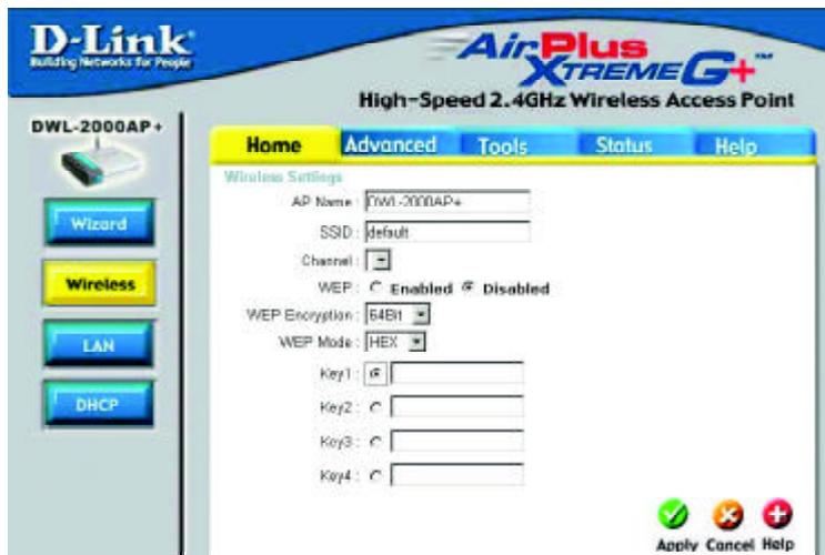
**SSID-** Service Set Identifier (SSID) is the name designated for a specific wireless local area network (WLAN). The SSID's factory default setting is **default**. The SSID can be easily changed to connect to an existing wireless network or to establish a new wireless network.
