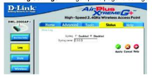
When you click on **Log Settings** in the previous window, the window at left appears. Select **Enabled** to save the log. In the **Syslog Server** field, input the IP Address of the computer on the network to which you wish to save the log settings. Click **Apply** to save the changes.
