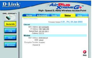
This page displays the current information about the DWL-2000AP+, such as the assigned IP Address and the wireless settings.
