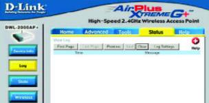
The Log keeps a running log of events and activities occurring on the Access Point. If the device is rebooted, the logs are automatically cleared. You may save the log files under Log Settings.
