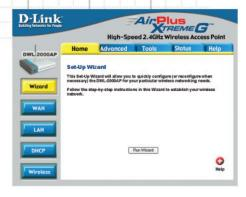
The Web-based configuration interface of the DWL-2000AP allows you to reconfigure the AP in any one of its four operating modes (see left); as well as to apply other management settings.
